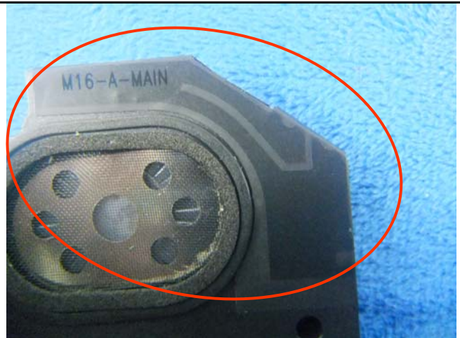
GSM/PCS/UMTS-FDD Antenna View
