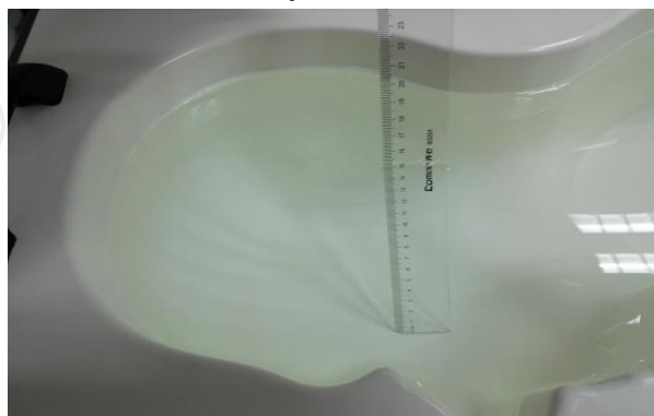
The Head Liquid of 2600MHz (15.1cm)
