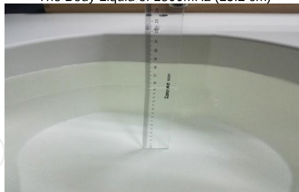
The Body Liquid of 2450MHz (15.3cm)
