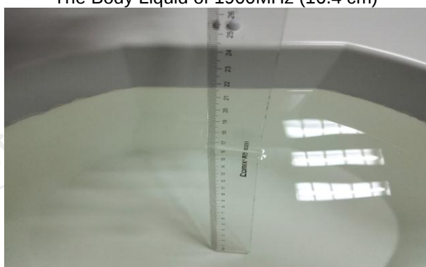
The Body Liquid of 2600MHz (16.5cm)
