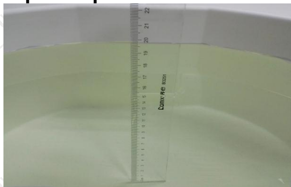
The Body Liquid of 835MHz (15.4cm)
