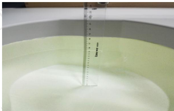
The Body Liquid of 1800MHz (15.2 cm)
