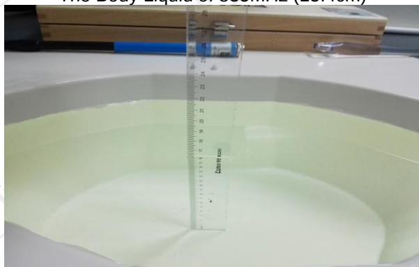
The Body Liquid of 1900MHz (16.4 cm)
