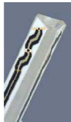
Figure 2.3 Probe Thick-Film Technique
