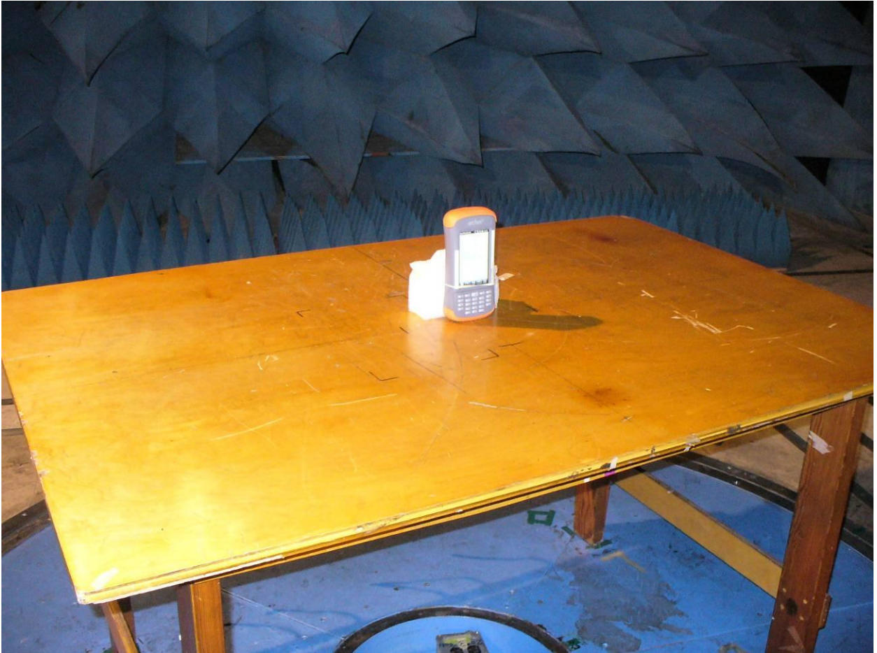
Figure 5: Radiated Emissions – Front View – (YZ Plane)
