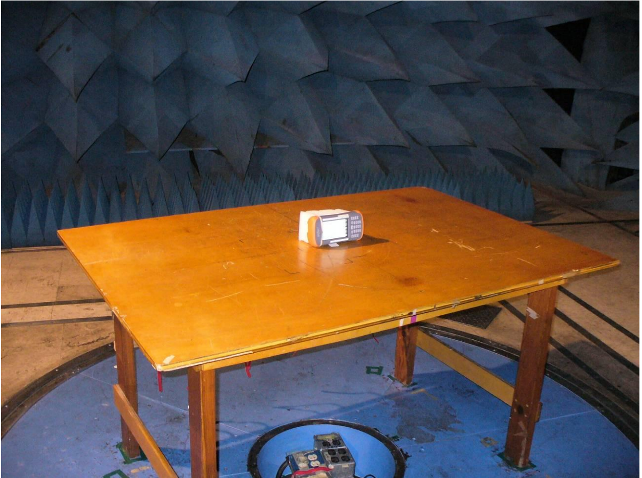
Figure 3: Radiated Emissions – Front View - (XY Plane)
