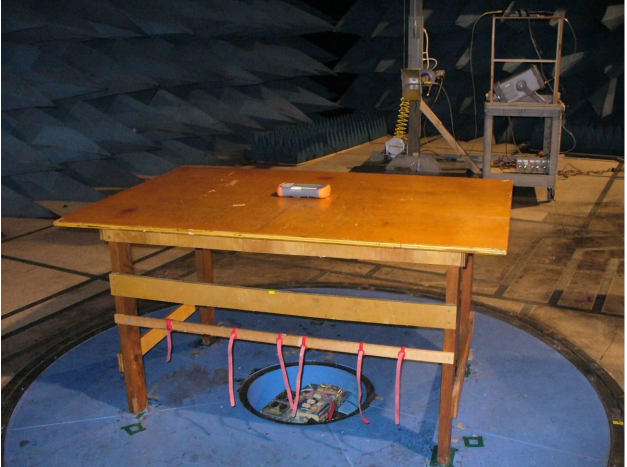
Figure 2: Radiated Emissions – Back View - (XZ Plane)
