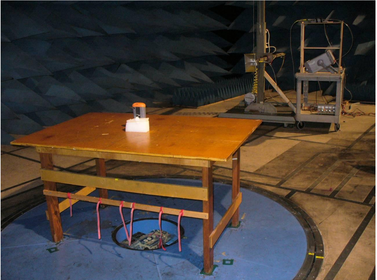
Figure 6: Radiated Emissions – Back View– (YZ Plane)
