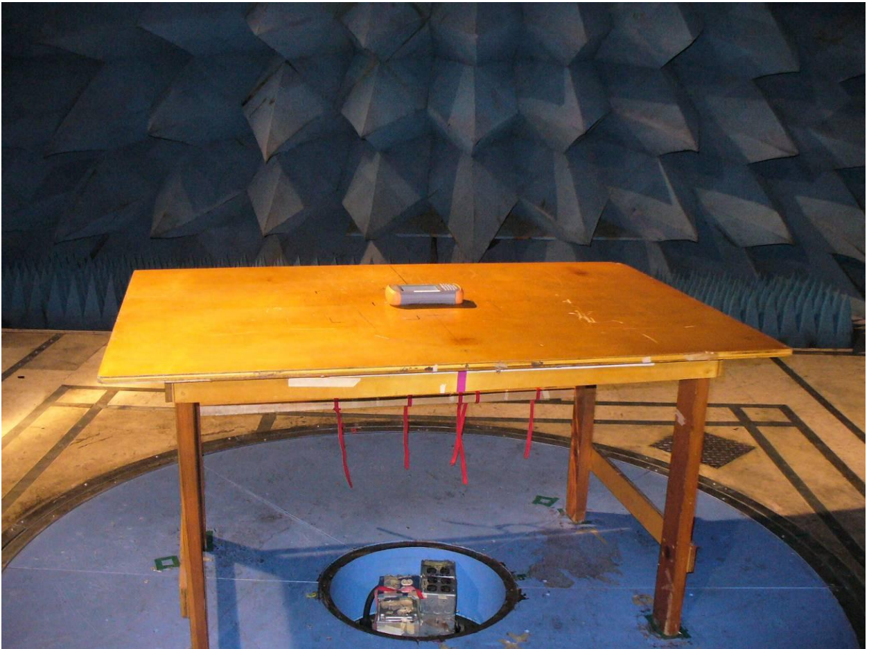
Figure 1: Radiated Emissions – Front View (XZ Plane)
