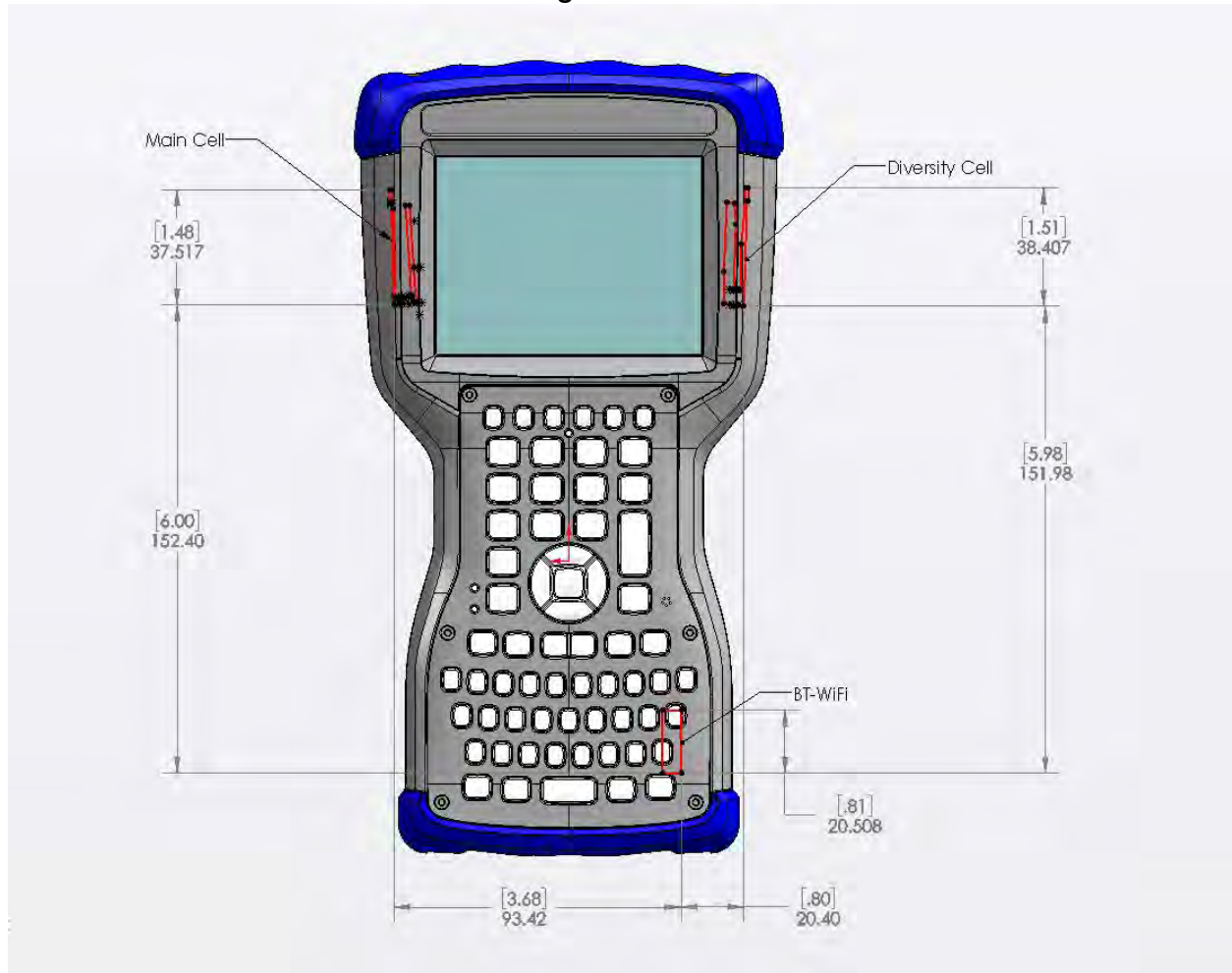
Figure 9.1 SAR Location Diagram of Antenna Distances
