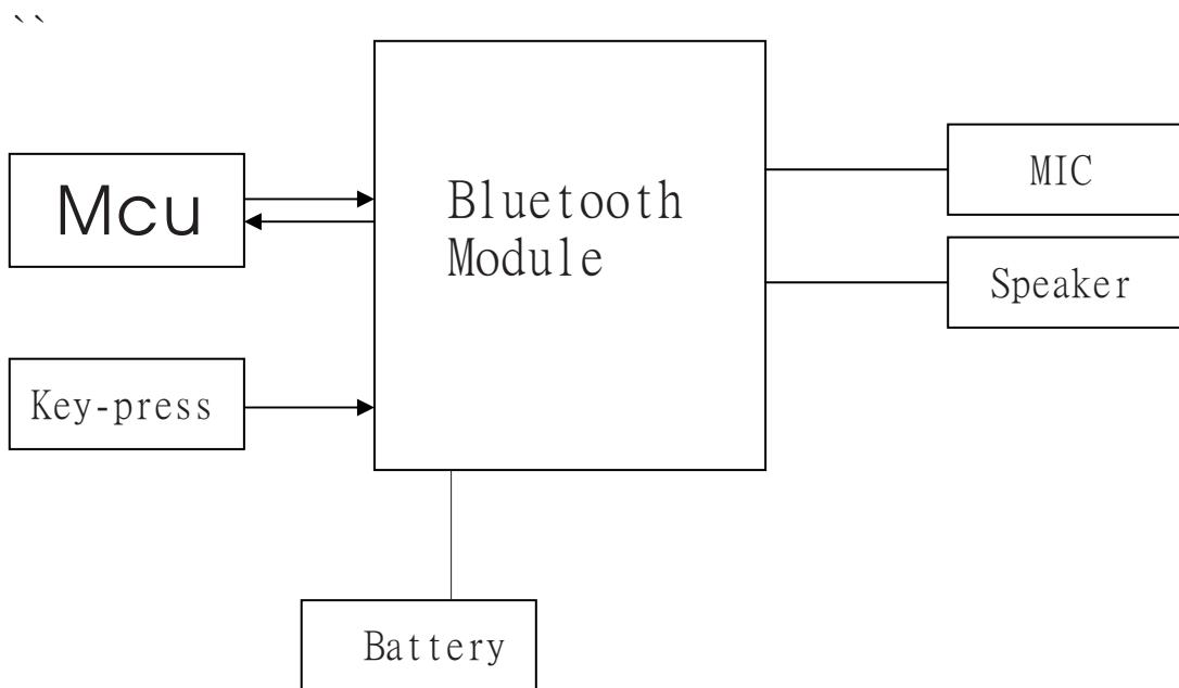
2. The Car radio adopt a BLUETOOTH module use short-range wireless communication Technology. The design applied is international identification ISM (Industrial Scientific and Medical) frequency bandwidth environment that is 2.4GHz ~ 2.48GHz bandwidth.
