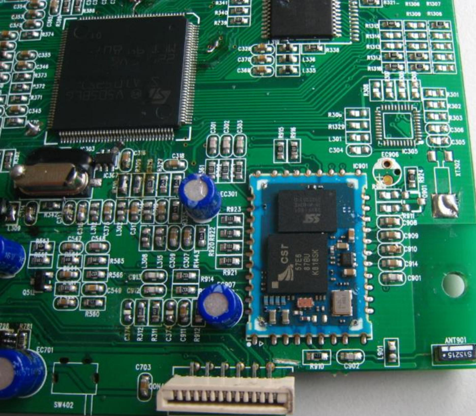
the antenna connection on PCB location
