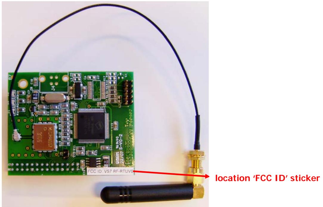
The 'FCC ID' sticker is located on the bottom right side of the RTU+® V6 RF module.
