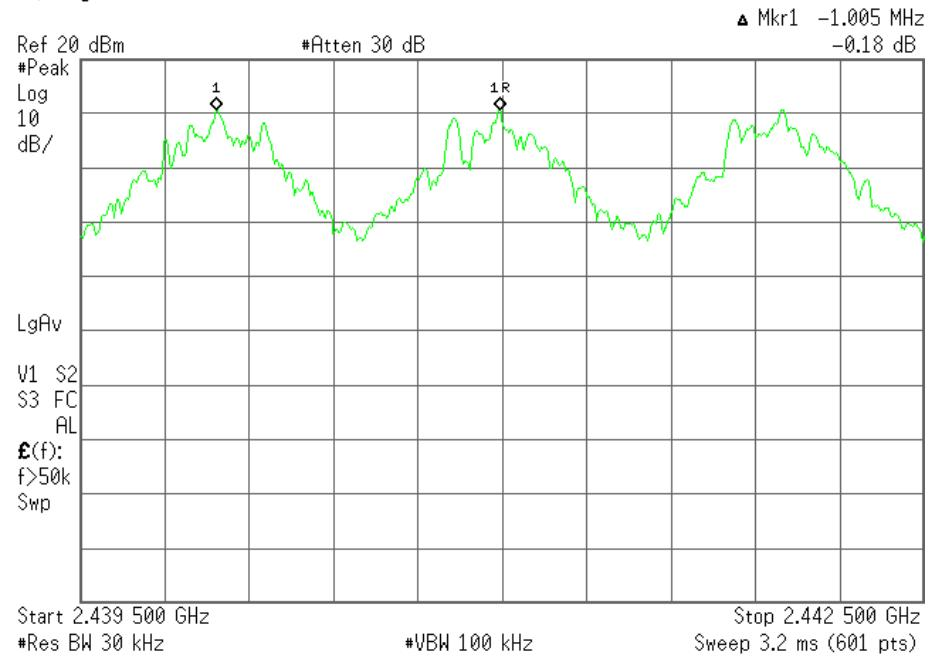
The hopping channel carrier frequencies are separated by a minimum of the 20 dB bandwidth of the hopping channel.
