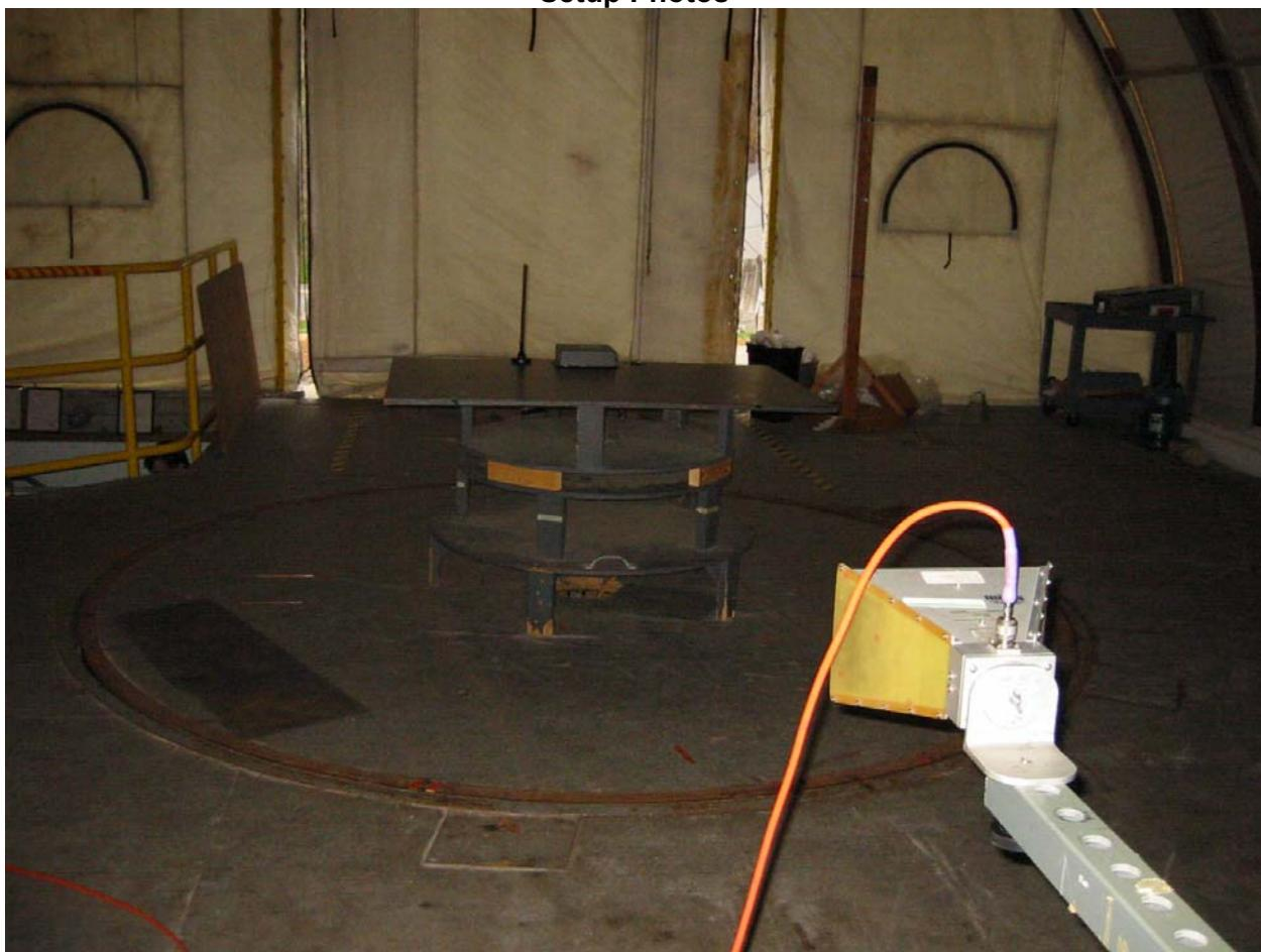
**Test Results:** Pass**Test Standard:** FCC Part 15 Subpart C**Test:** RF Output Power, FCC §15.247(b)(3)**Performance Criterion:** Conducted RF Output Power must not exceed 1 Watt (30 dBm). EIRP must not exceed 4 Watts (36 dBm).**Test Environment:**
