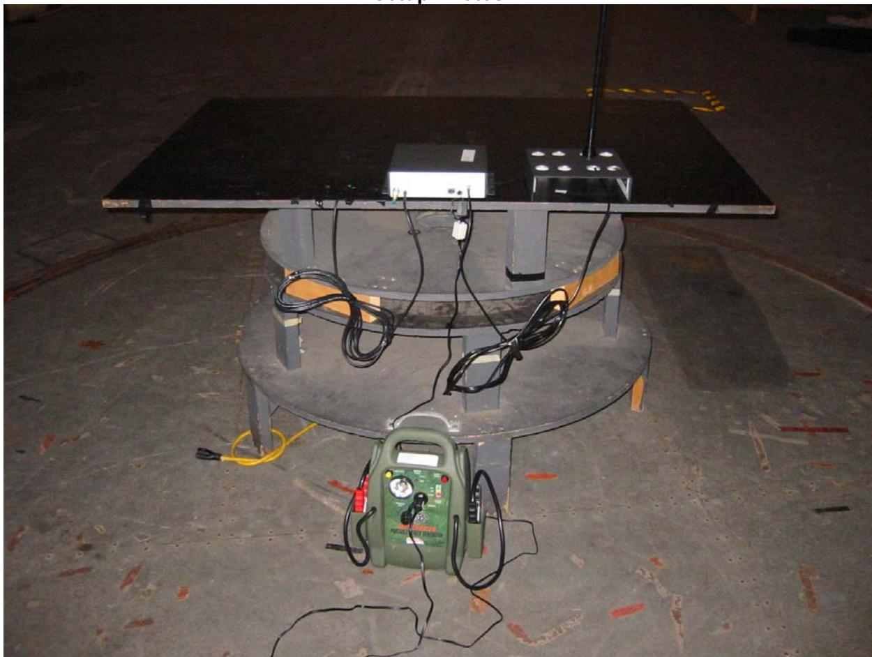
**Test Results:** Pass**Test Standard:** FCC Part 22, FCC Part 74, FCC Part 90**Test:** RF Output Power, FCC §22.565(a), FCC §74.861(d)(1), FCC §90.205(d)**Performance Criterion:** Power must not exceed the following values:
