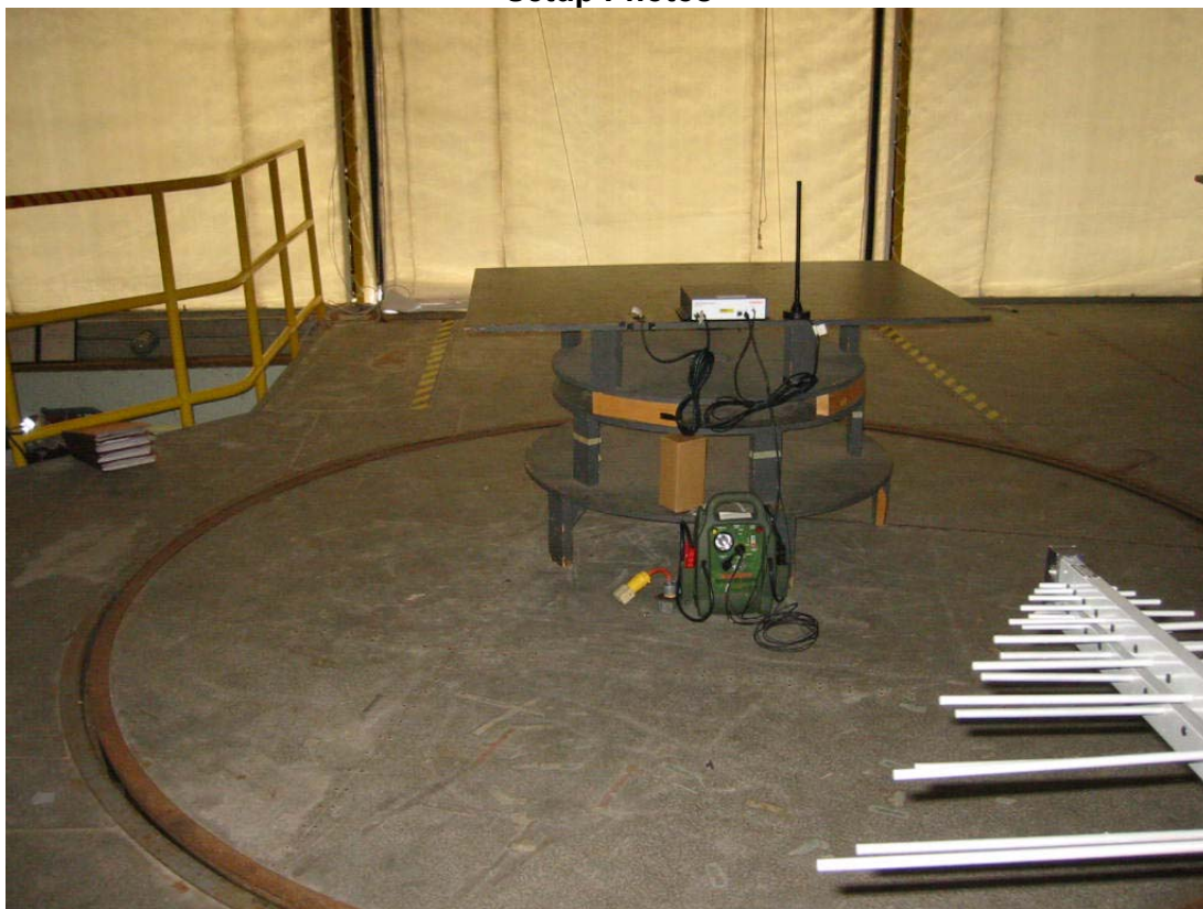
30-1000 MHz Radiated Emissions
