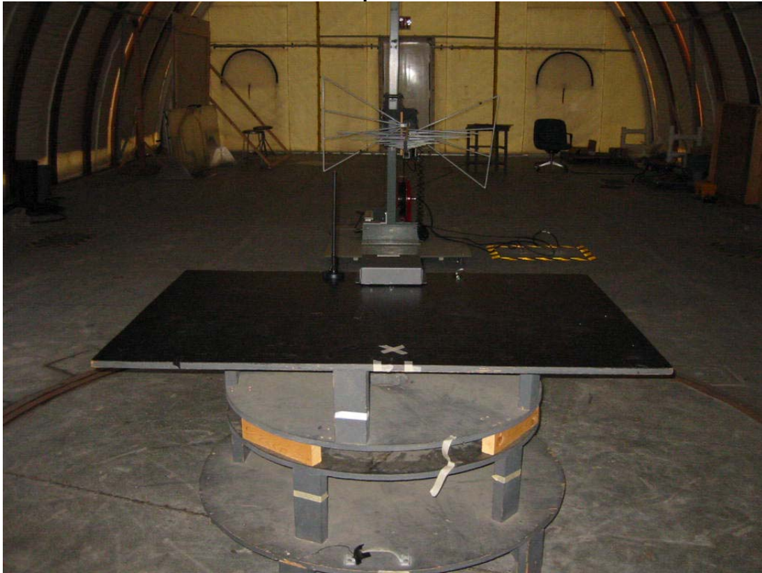
30-1000 MHz Radiated Emissions
