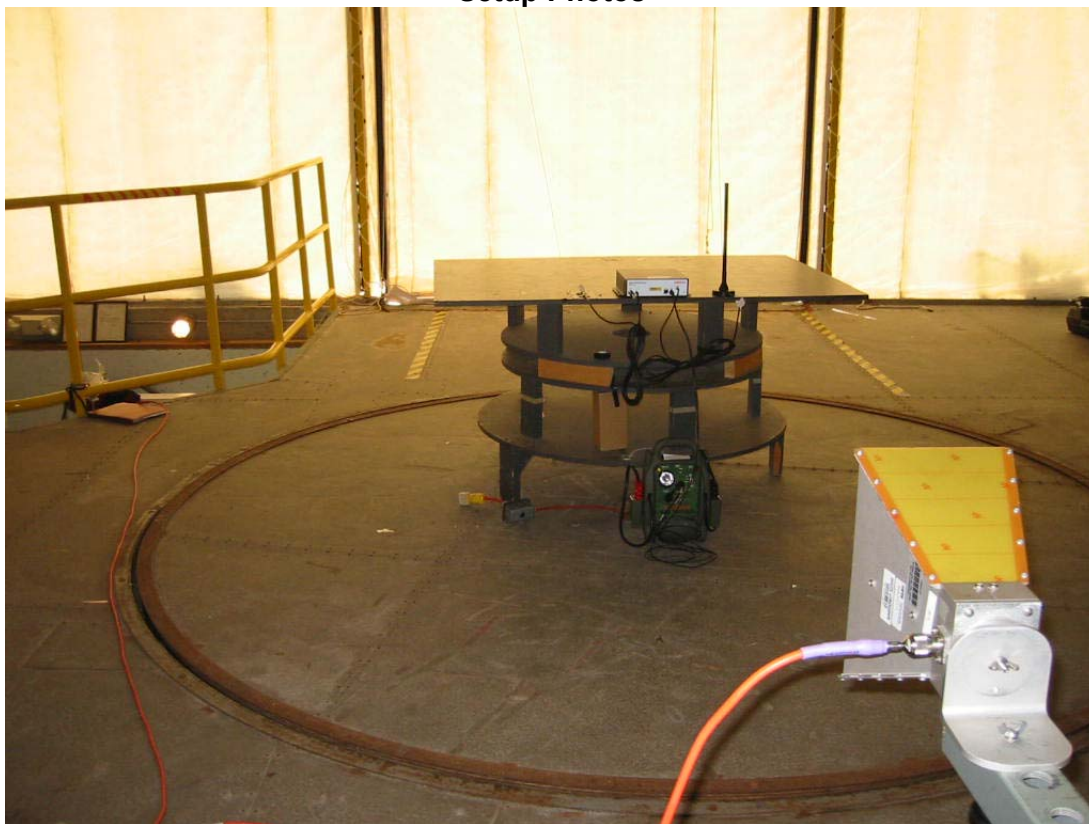
1-9 GHz Radiated Emissions
