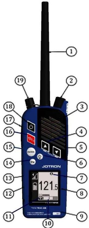
Figure 3 Tron TR30 AIR components
