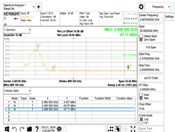
Spurious Emission_BLE 1M_LowCH00-2402MHz
