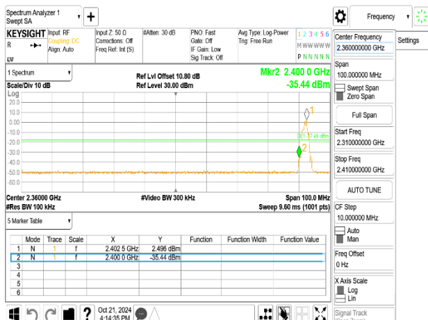
Band Edge_BLE 2M_LowCH00-2402MHz
