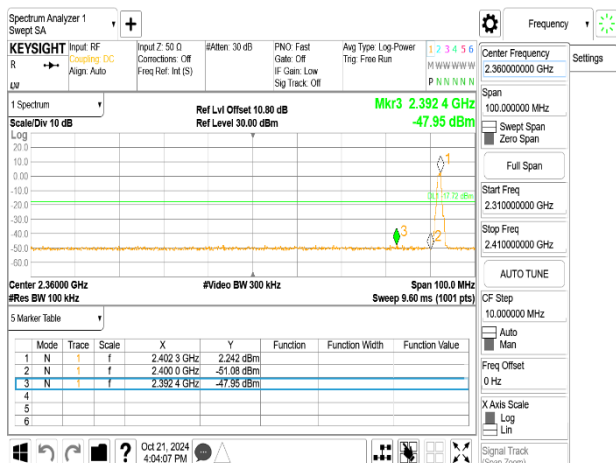
Band Edge_BLE 1M_HighCH39-2480MHz
