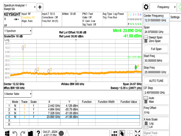
Spurious Emission_BLE 1M_MidCH20-2442MHz
