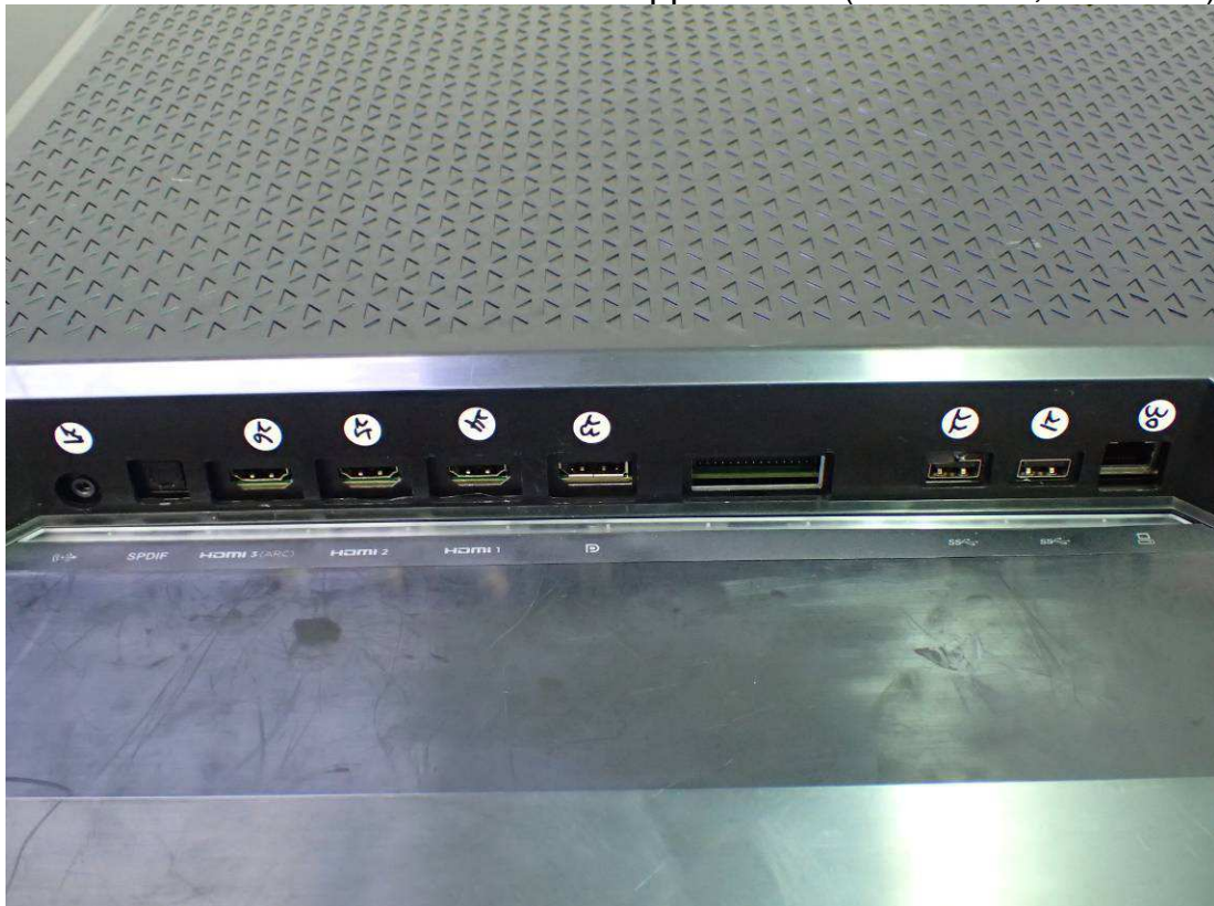
Figure 6 General Appearance (Back View, I/O Ports)
