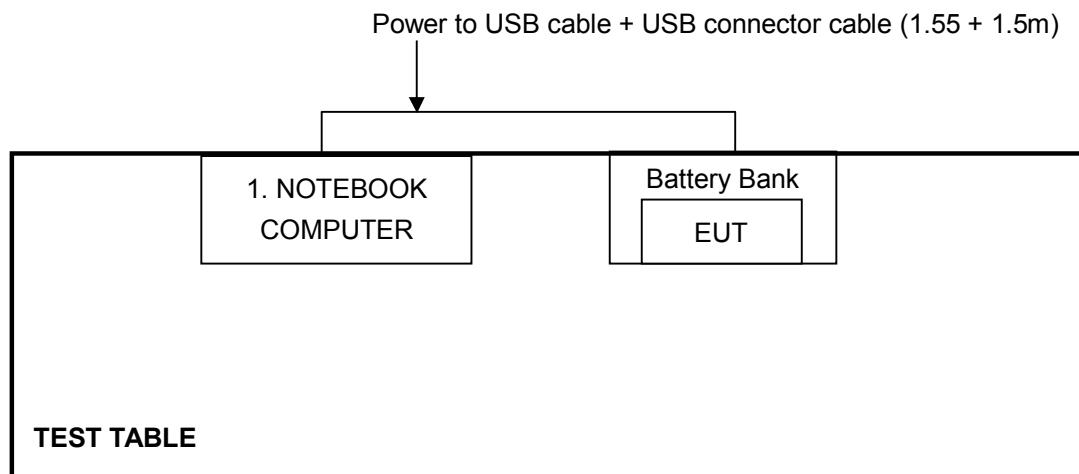
**For Battery Bank + Power to USB cable + USB connector cable Adapter Mode :**
