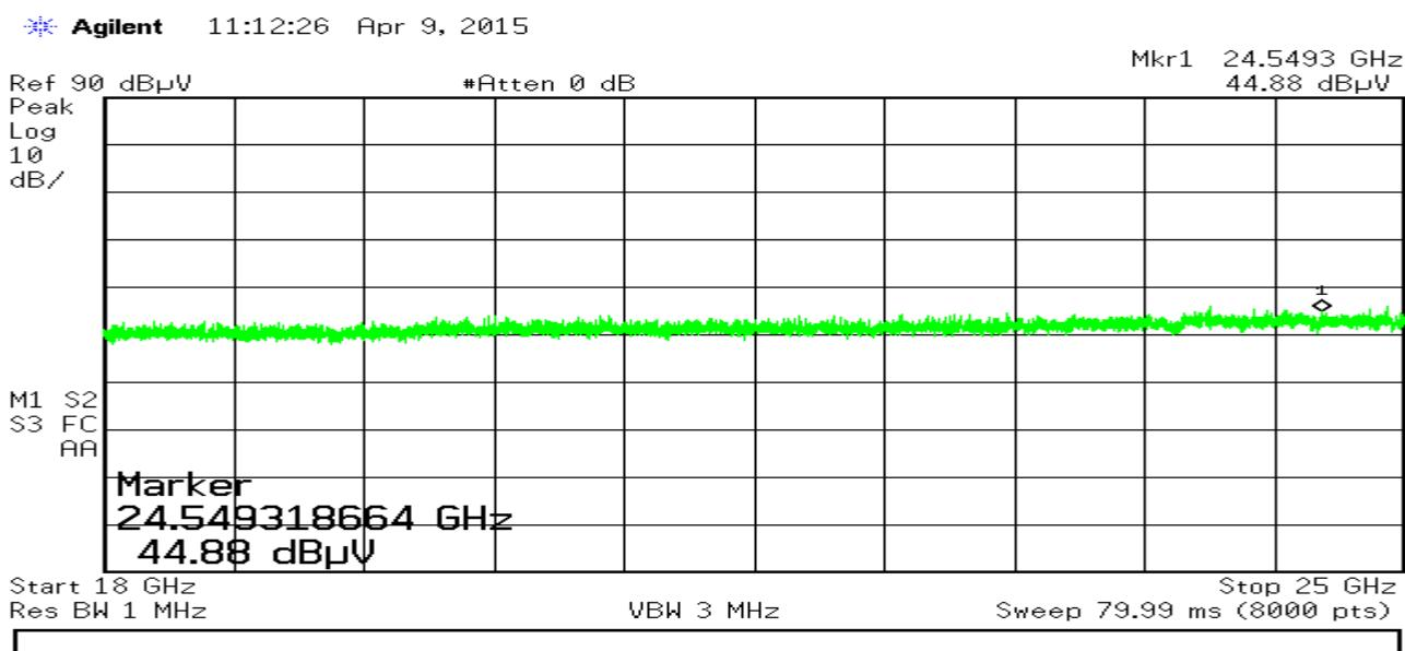
**Radiated Emissions – 18 GHz to 24 GHz – Vertical:**
