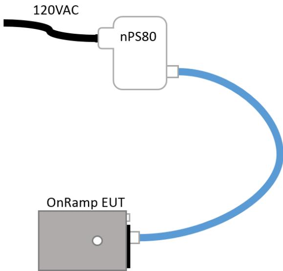
Note: the nPS80 is a power module used to simulate a typical host device providing power to the EUT.
