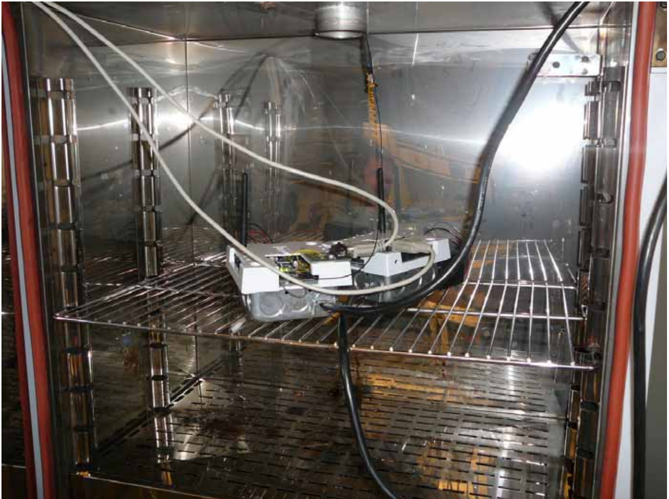
Figure 10 –Frequency Stability Test Setup – Temperature Chamber at +50°C
