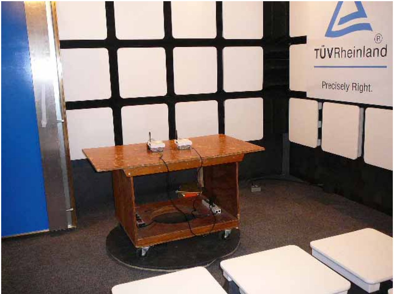
Figure 6 - Radiated Spurious Emissions Test Setup (Radiated Prescan- Semi Anechoic Chamber)
