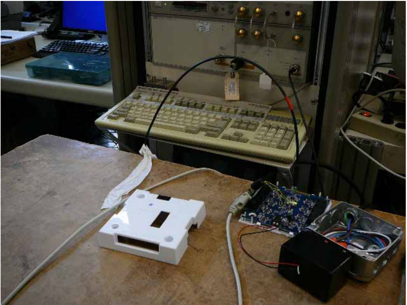
Figure 3 - Radiated Emissions Test Setup (Semi-Anechoic Chamber 2)
