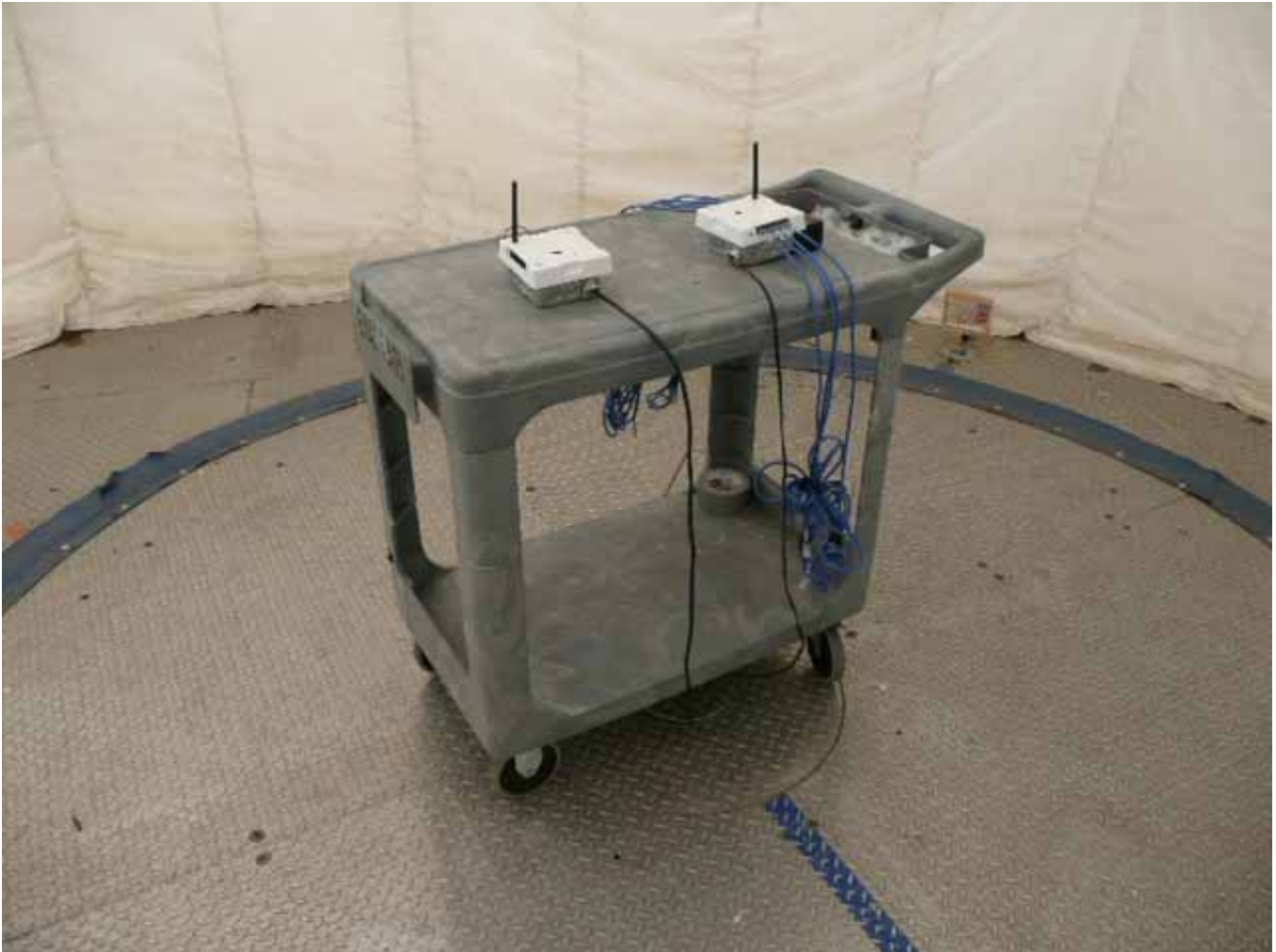
Figure 7 - Radiated Spurious Emissions Test Setup (Radiated Final Test - OATS)
