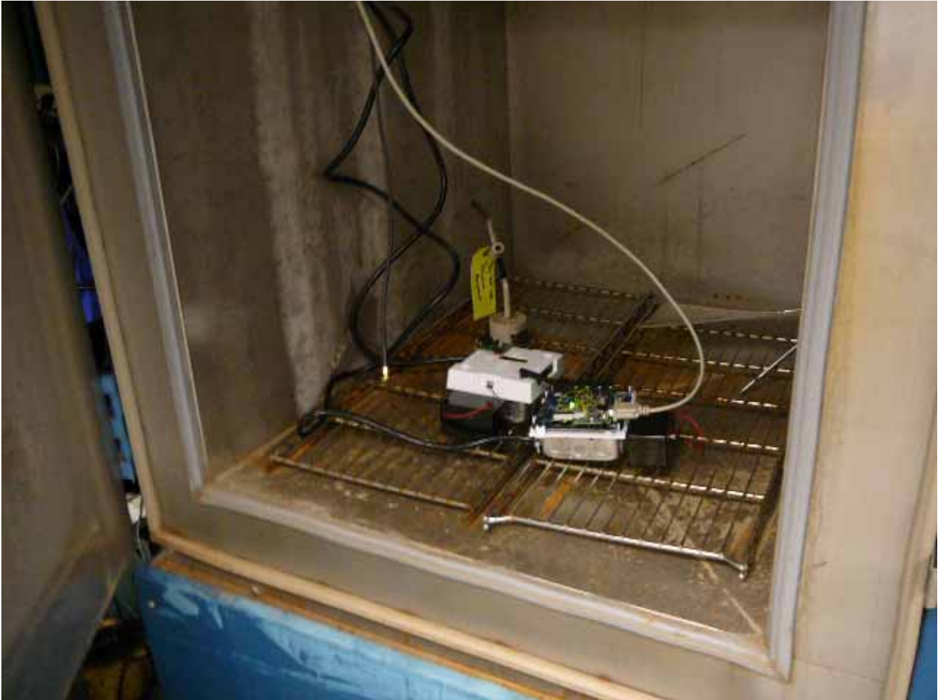
Figure 11 –Frequency Stability Test Setup – Humidity Chamber at 0°C
