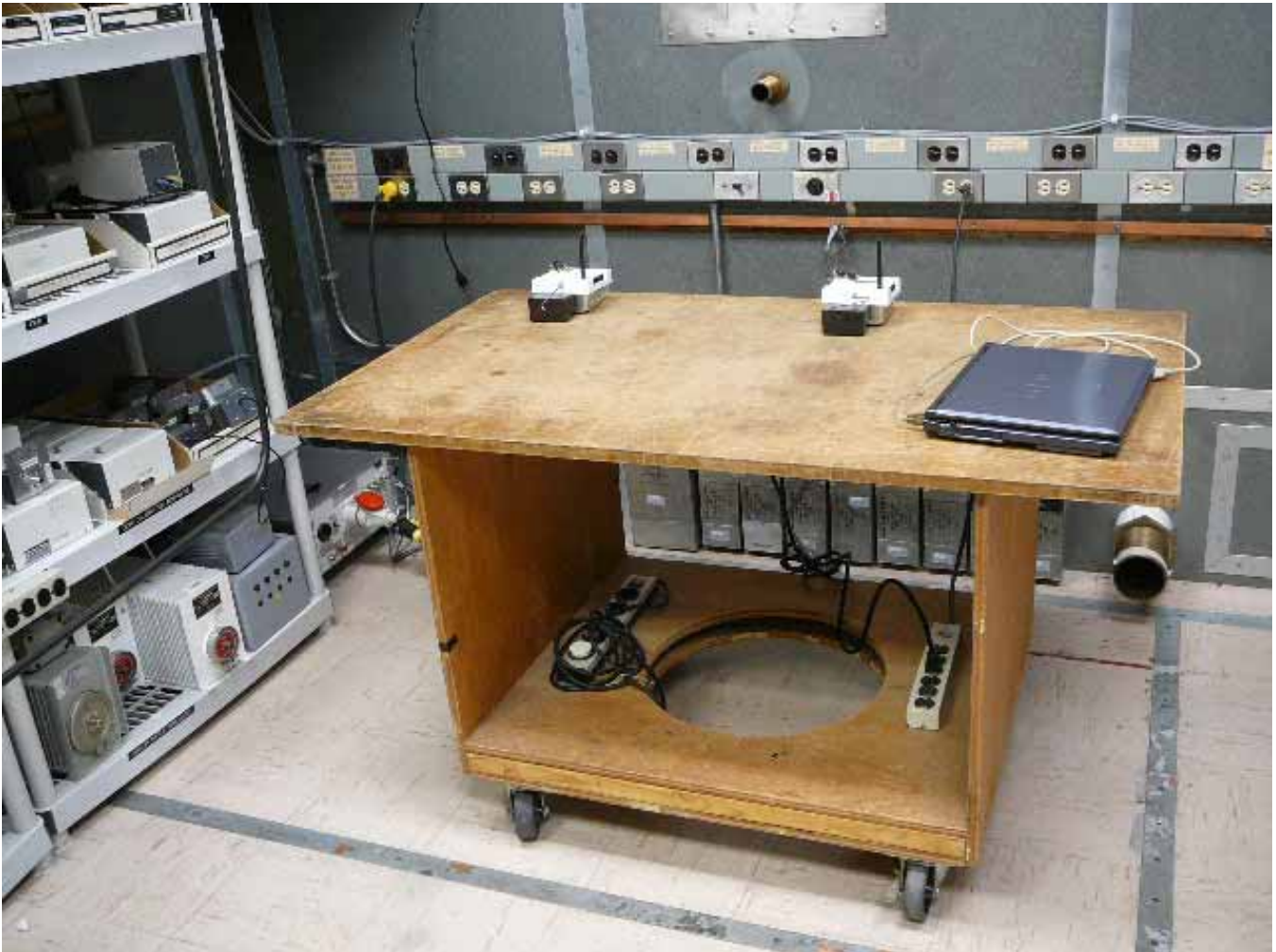
Figure 9 –Conducted Emissions Test Setup
