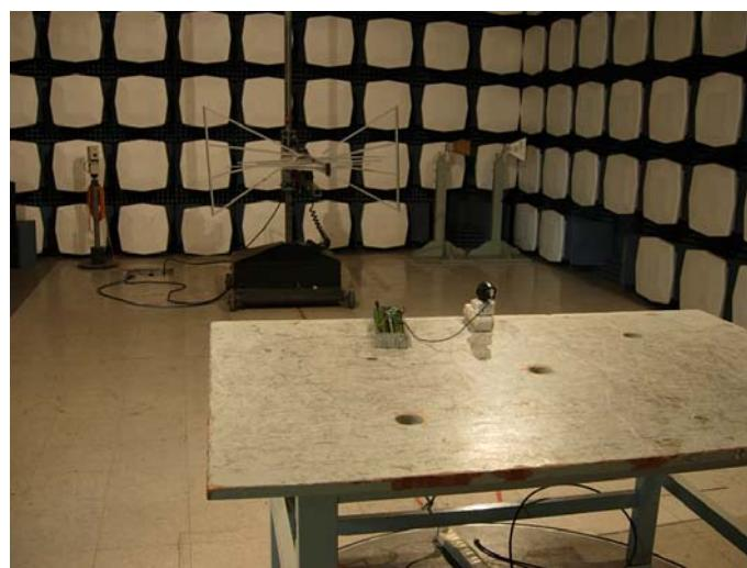
*Maximized Radiated Emission Test Set-up - Horizontal Polarization*
