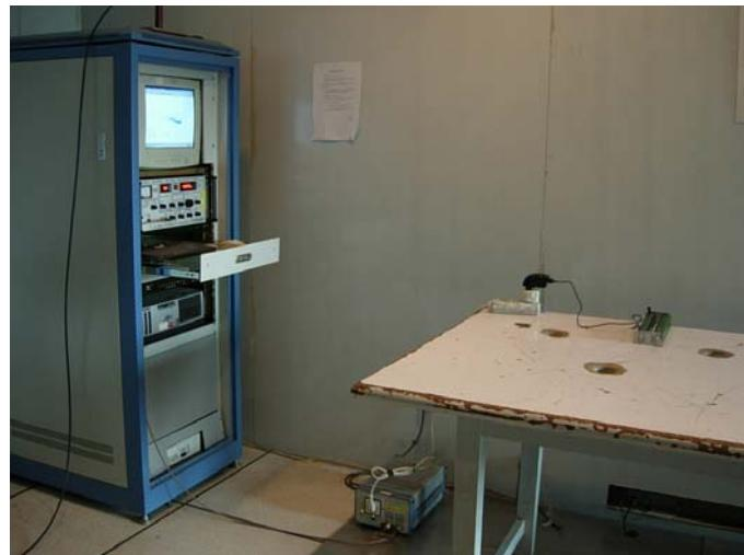
*Maximized Conducted Emission Test Set-up*
