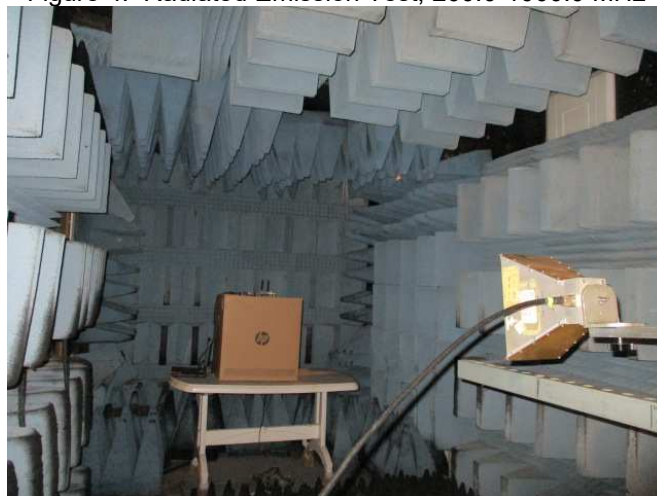
Figure 5. Radiated Emission Test, 1.0-18.0 GHz
