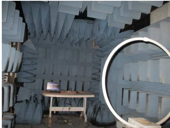
Figure 2. Radiated Emission Test, 0.009-30.0 MHz
