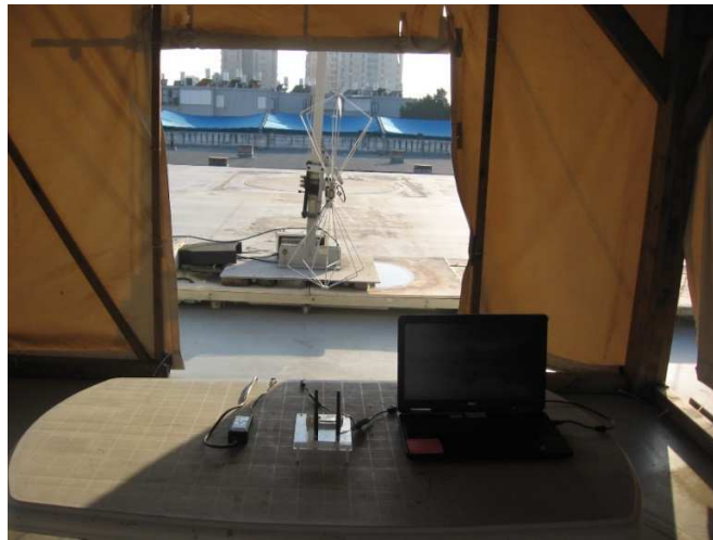
Figure 3. Radiated Emission Test, 30.0-200.0 MHz
