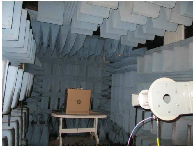
Figure 6. Radiated Emission Test, 18-26.5 GHz
