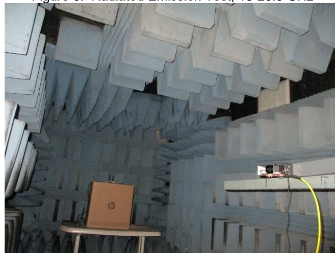
Figure 7. Radiated Emission Test, 26.5-40.0 GHz
