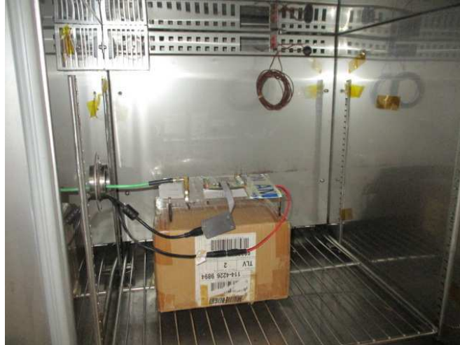
Figure 1. Conducted Emission Test (with Spectrum Analyzer)
