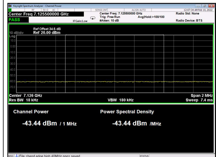
Figure 37 Higher Band Edge, 20MHz BW
