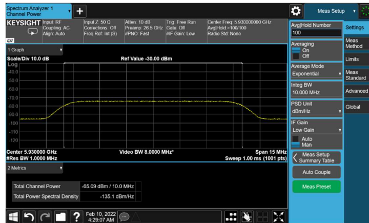
Figure 69. AWGN signal at 5930MHz
