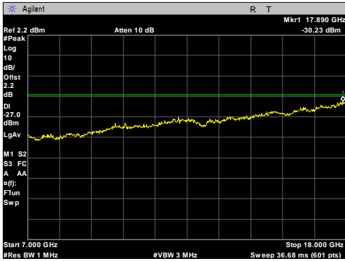
Plot 70. Radiated Spurious Emissions, Low Channel, 40 MHz, 7 GHz – 18 GHz
