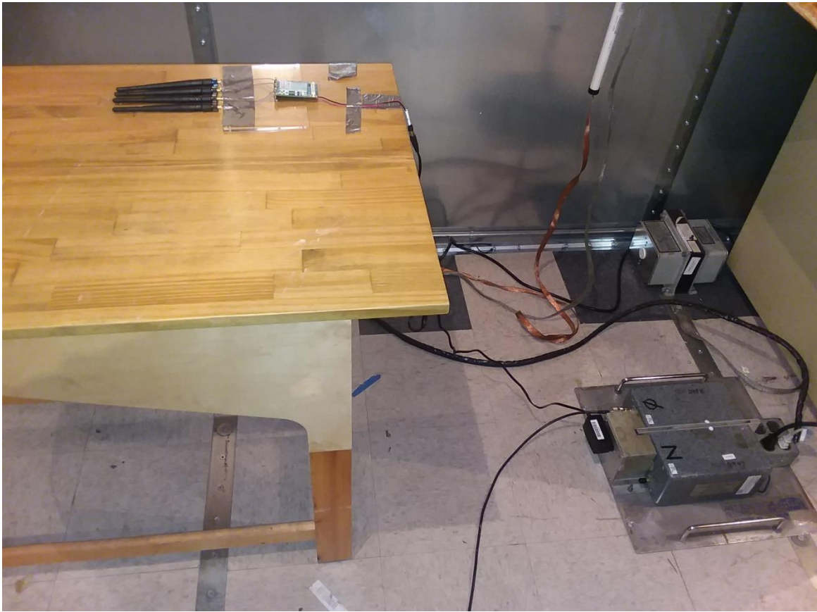
Photograph 5. Conducted Emissions, Test Setup
