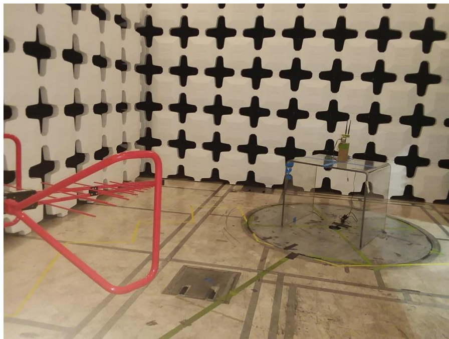
Photograph 4. Radiated Emissions, 2x2 Test Setup Below 1GHz
