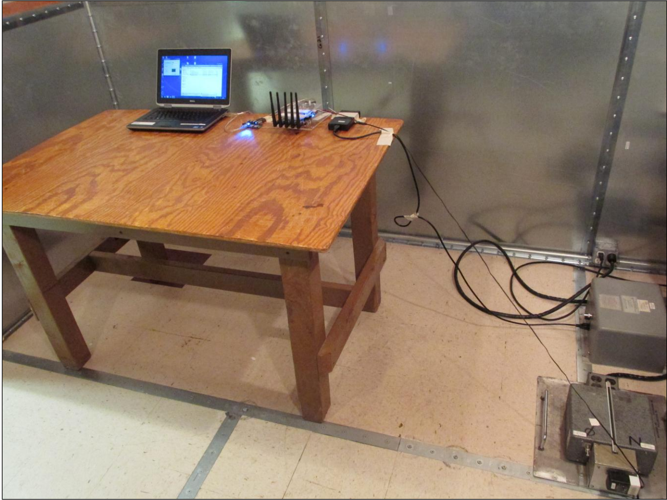
Photograph 3. Conducted Emissions, Test Setup
