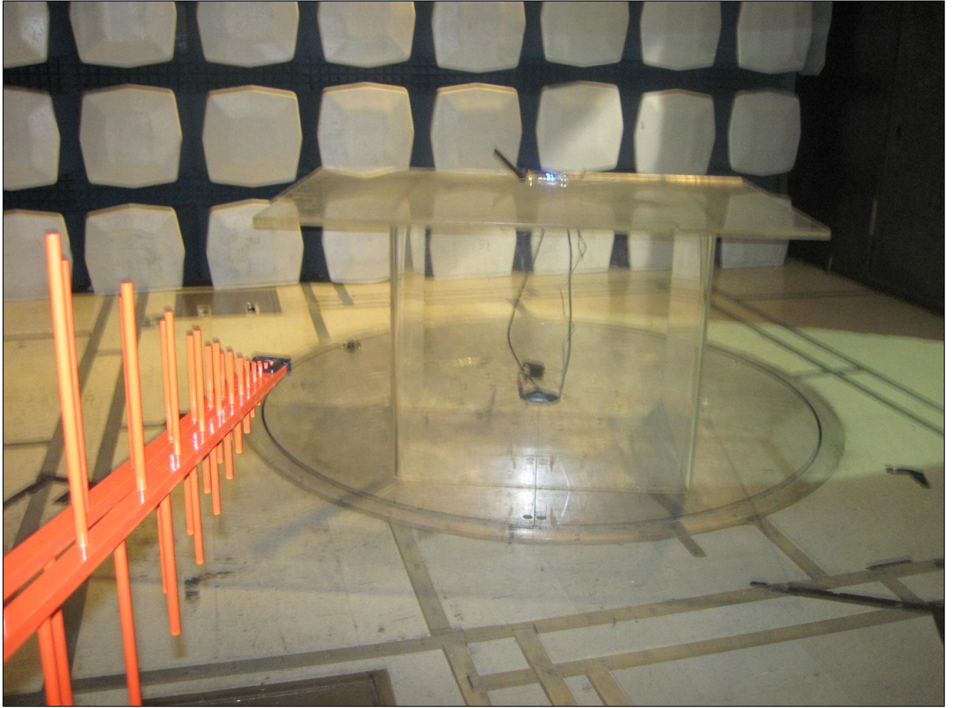
Photograph 2. Radiated Emission, Test Setup
