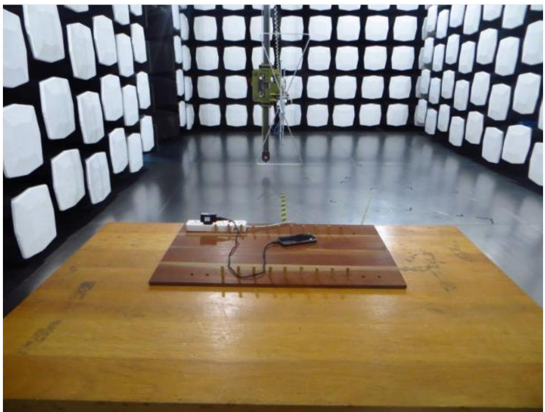
6. Part 15B Radiated emission (charger1) above 1GHz
