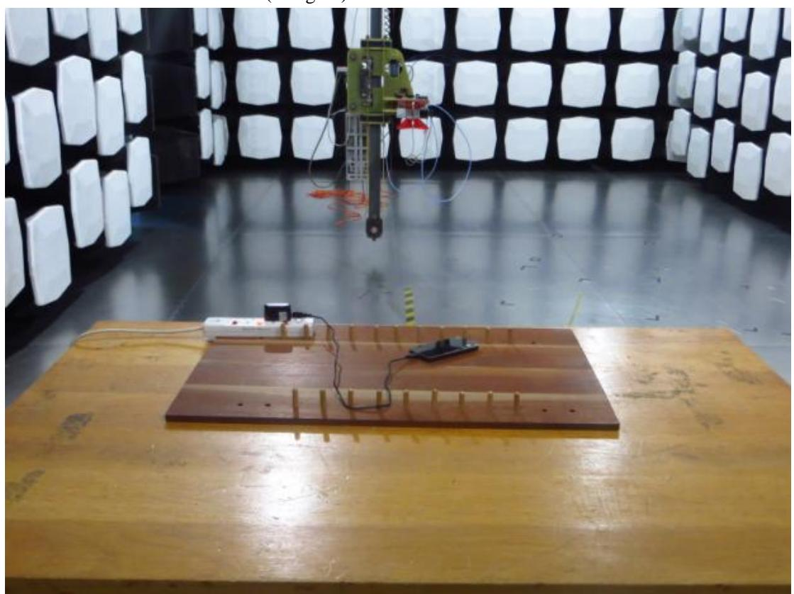
7. Part 15B Radiated emission (charger2) above 1GHz
