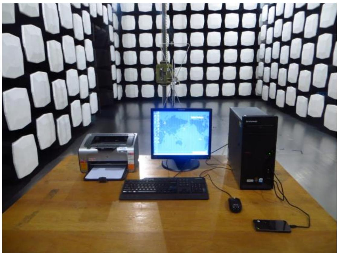
9. Part 15B Radiated emission (USB) above 1GHz
