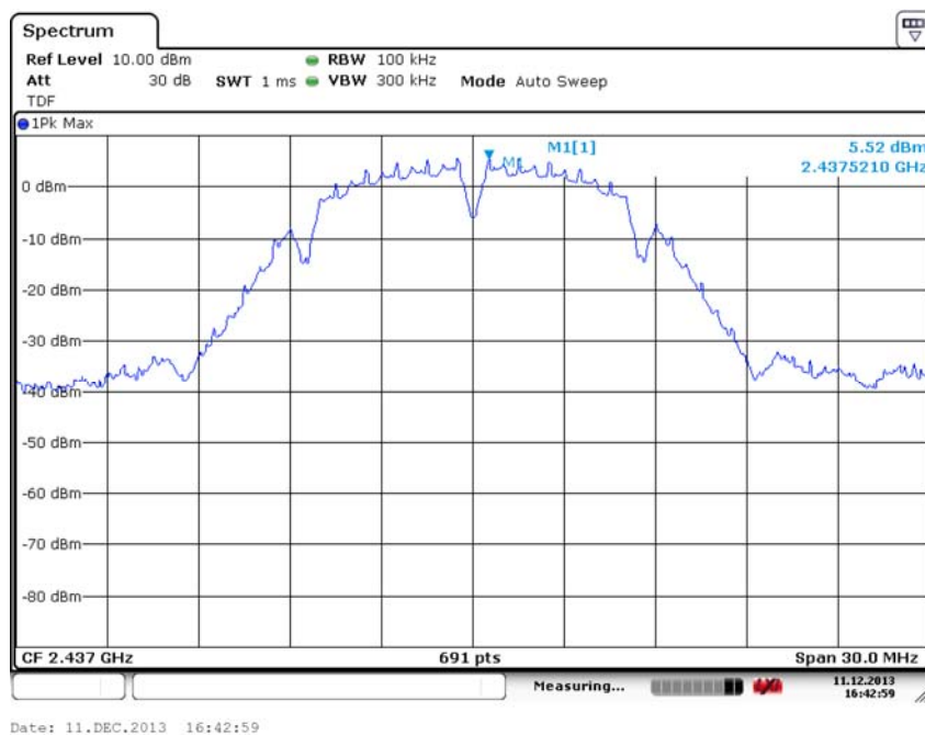
Fig. 36 Conducted Spurious Emission (802.11b, Ch6, Center Frequency)
