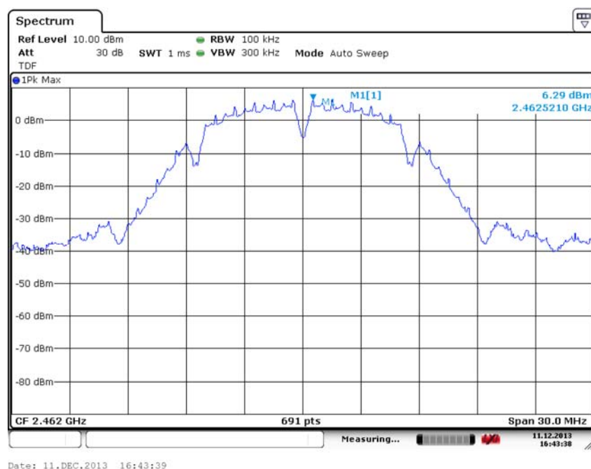
Fig. 39 Conducted Spurious Emission (802.11b, Ch11, Center Frequency)
