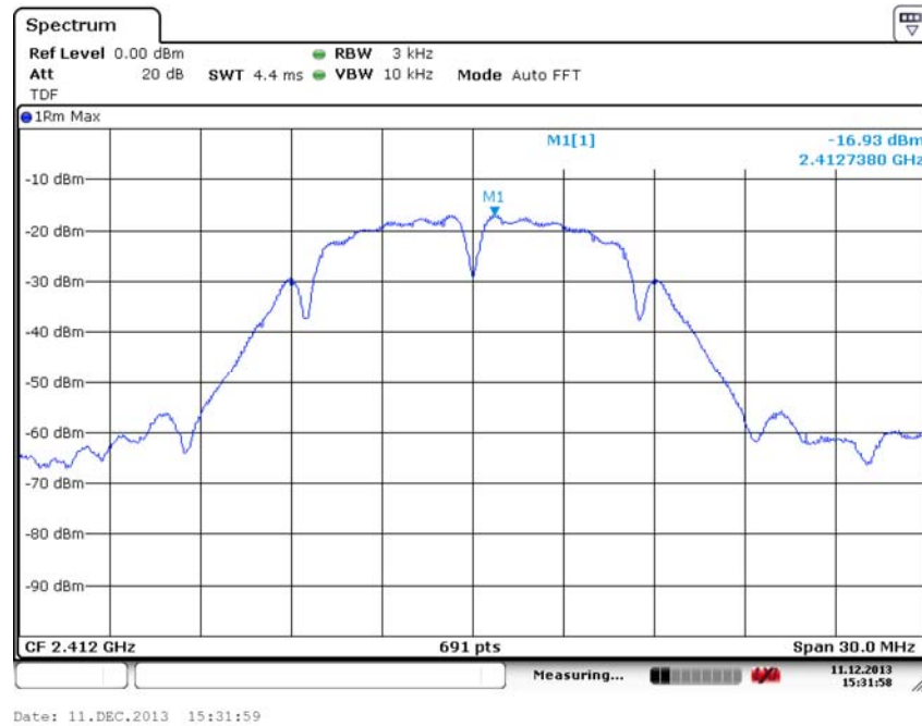
Fig. 1 Power Spectral Density (802.11b, Ch 1)
