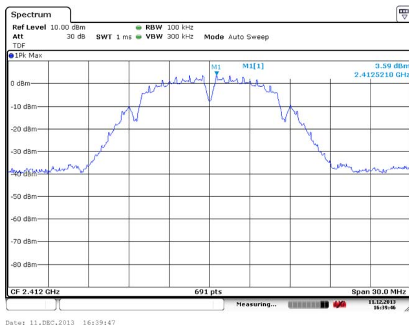
Fig. 33 Conducted Spurious Emission (802.11b, Ch1, Center Frequency)
