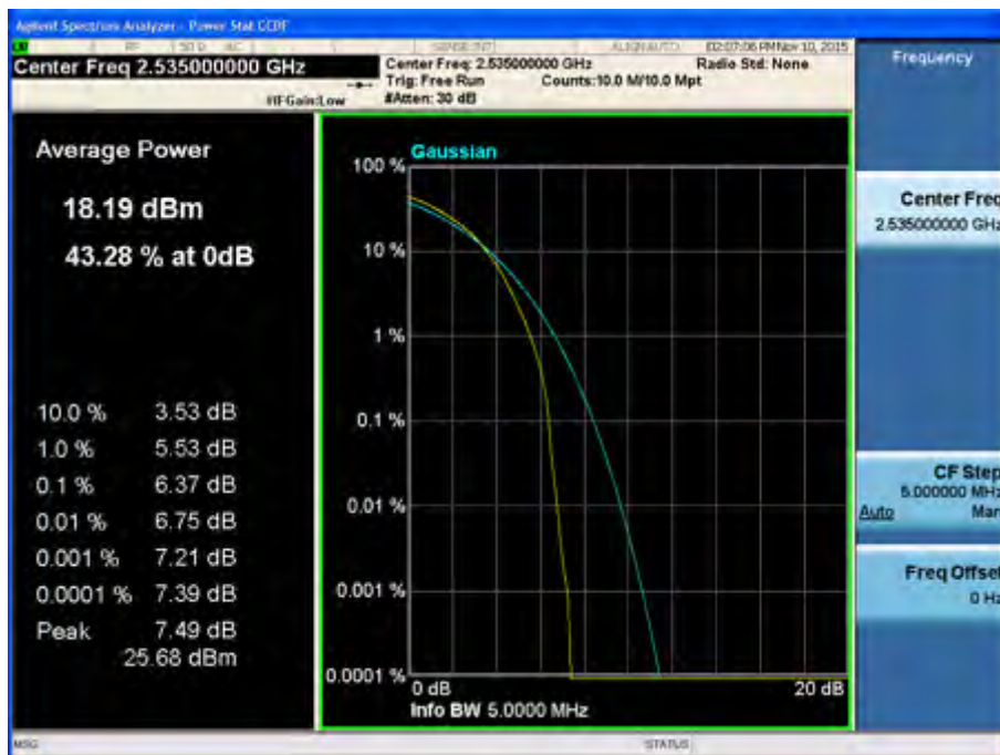
Peak-Average Ratio Plot (10 MHz BW, QPSK, Band 7 – Mid Channel)
