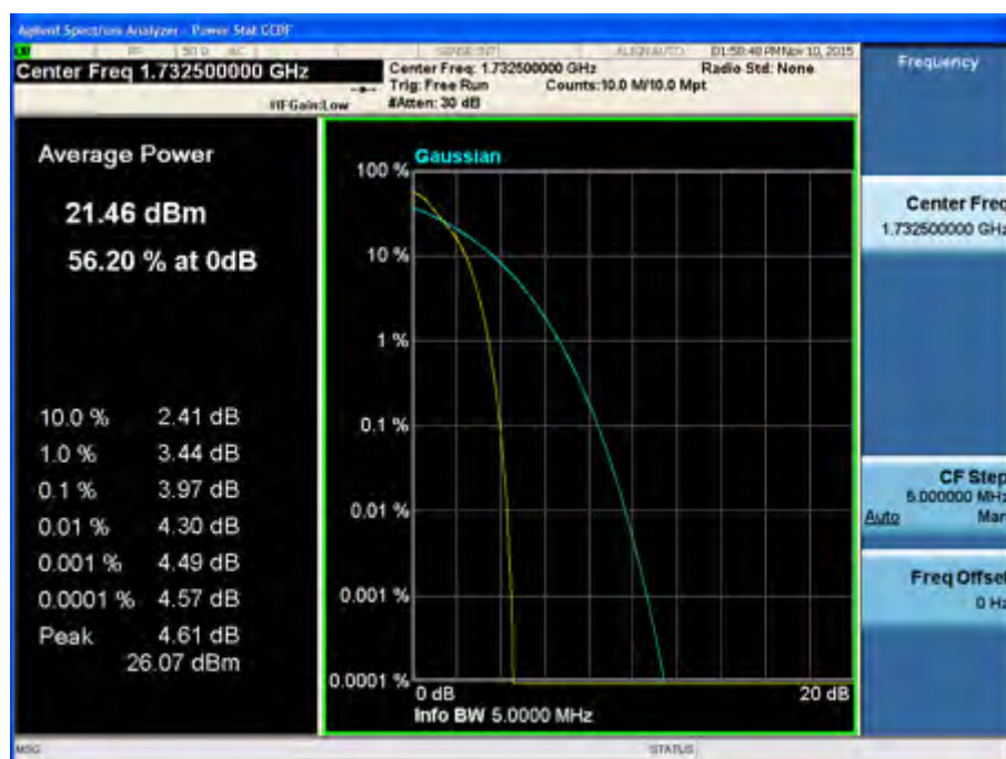
Peak-Average Ratio Plot (1.4 MHz BW, 16QAM, Band 4 – Mid Channel)
