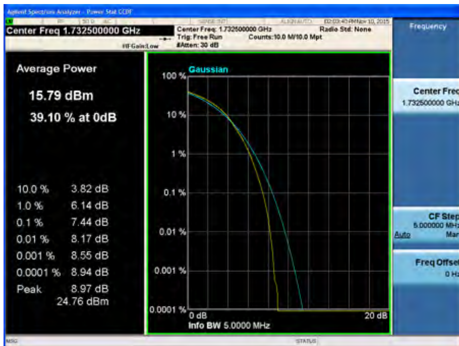
Peak-Average Ratio Plot (20 MHz BW, QPSK, Band 4 – Mid Channel)
