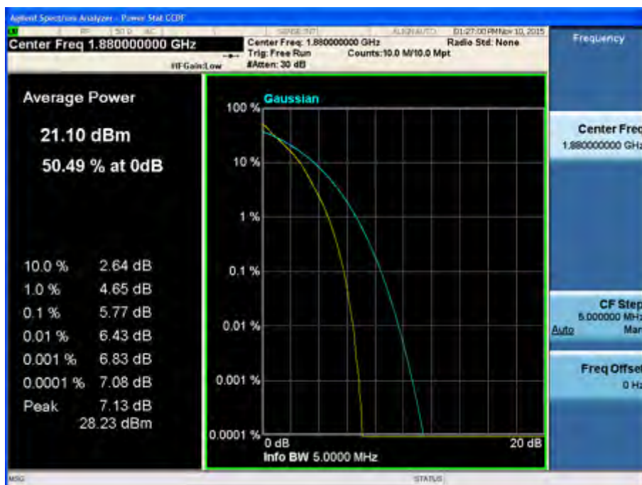
Peak-Average Ratio Plot (5 MHz BW, 16QAM, Band 2 – Mid Channel)
