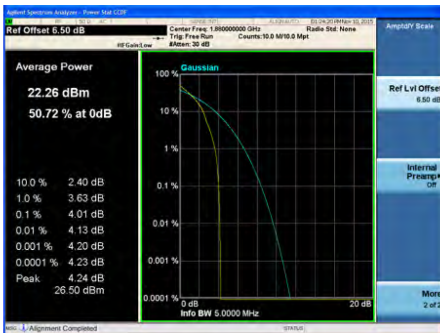
Peak-Average Ratio Plot (1.4 MHz BW, QPSK, Band 2 – Mid Channel)
