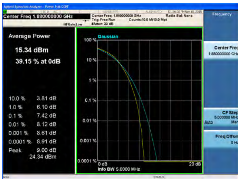
Peak-Average Ratio Plot (15 MHz BW, 16QAM, Band 2 – Mid Channel)
