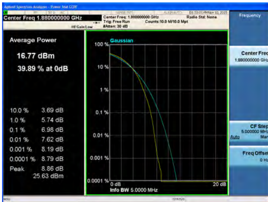
Peak-Average Ratio Plot (15 MHz BW, QPSK, Band 2 – Mid Channel)
