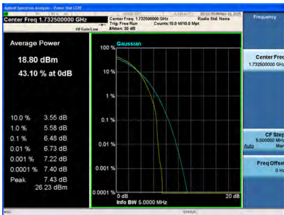
Peak-Average Ratio Plot (10 MHz BW, QPSK, Band 4 – Mid Channel)
