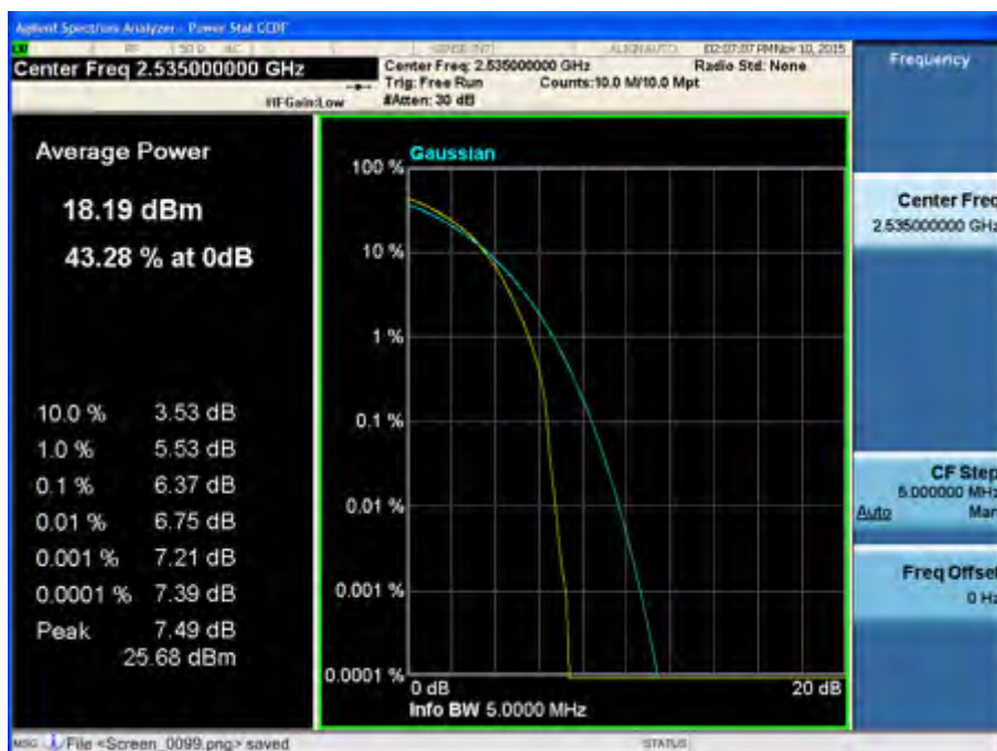
Peak-Average Ratio Plot (10 MHz BW, 16QAM, Band 7 – Mid Channel)
