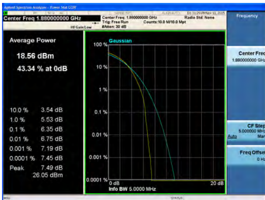
Peak-Average Ratio Plot (10 MHz BW, 16QAM, Band 2 – Mid Channel)
