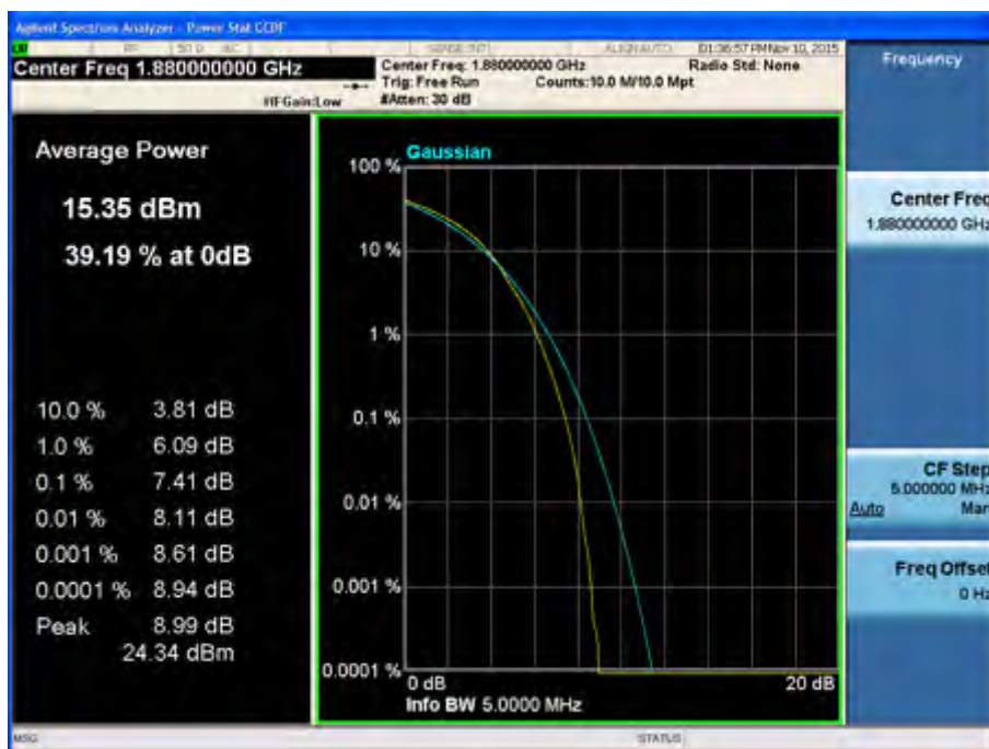
Peak-Average Ratio Plot (20 MHz BW, QPSK, Band 2 – Mid Channel)
