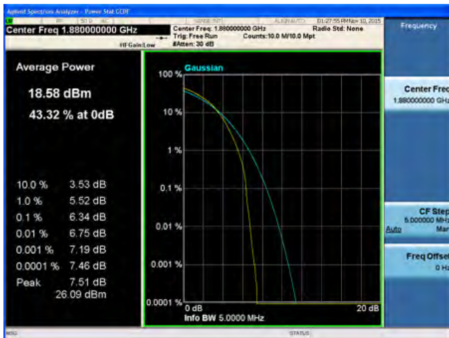
Peak-Average Ratio Plot (10 MHz BW, QPSK, Band 2 – Mid Channel)
