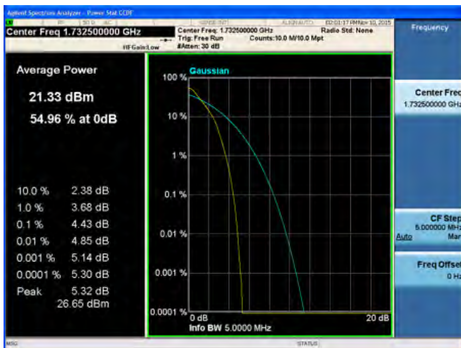
Peak-Average Ratio Plot (3 MHz BW, 16QAM, Band 4 – Mid Channel)
