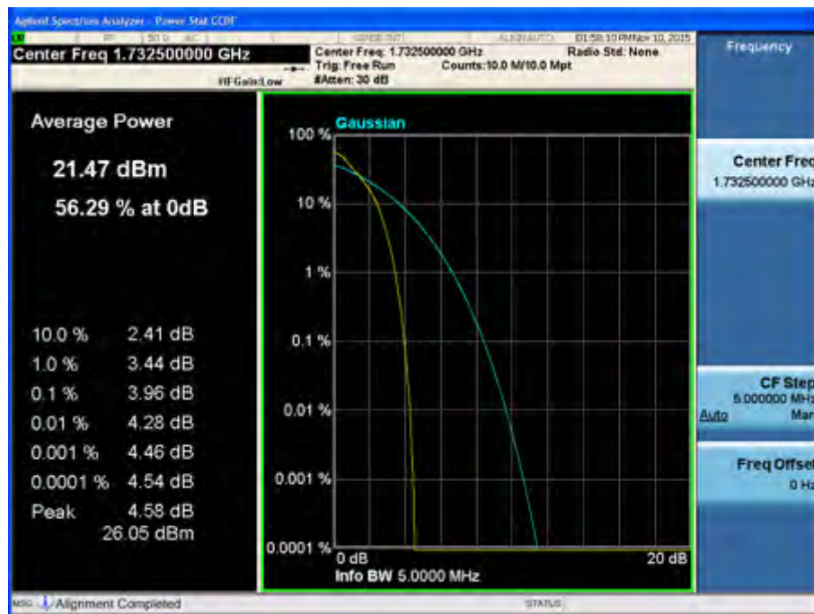
Peak-Average Ratio Plot (1.4 MHz BW, QPSK, Band 4 – Mid Channel)
