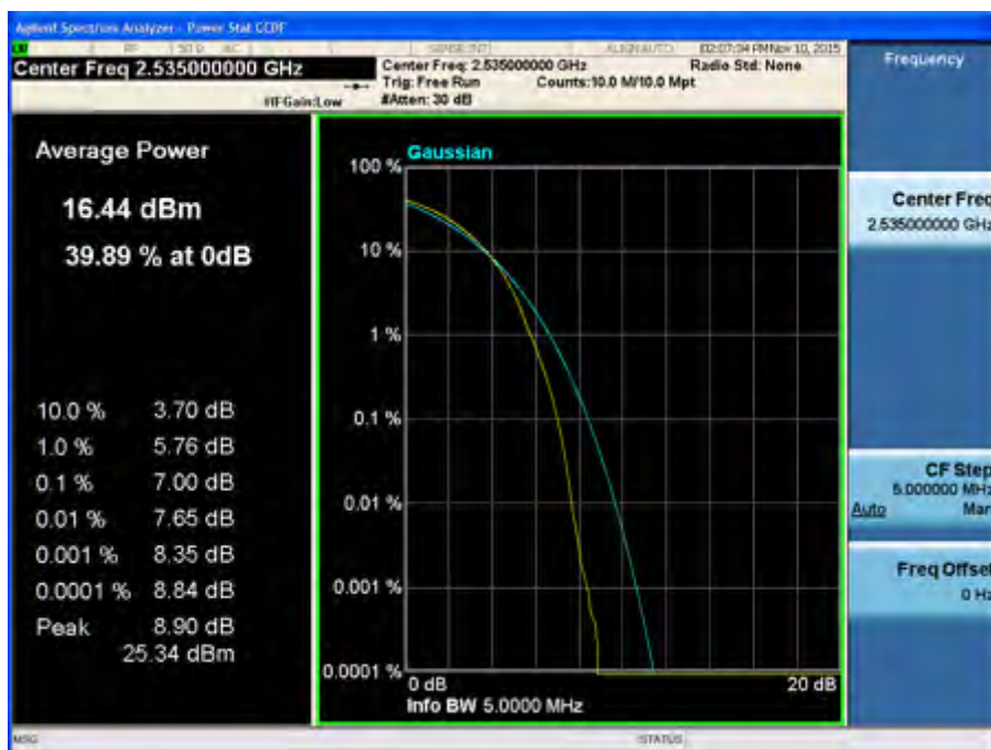
Peak-Average Ratio Plot (15 MHz BW, QPSK, Band 7 – Mid Channel)
