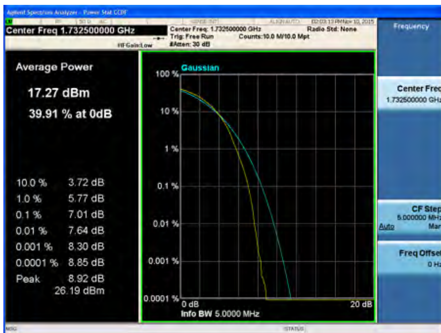
Peak-Average Ratio Plot (15 MHz BW, 16QAM, Band 4 – Mid Channel)
