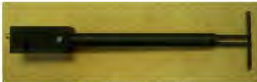
Figure 1 – MVG COMOSAR Validation Dipole
