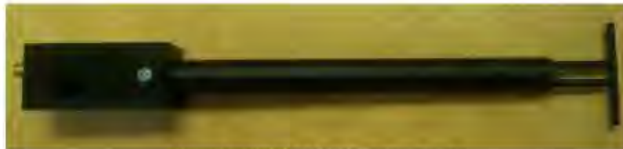
Figure 1 – MVG COMOSAR Validation Dipole
