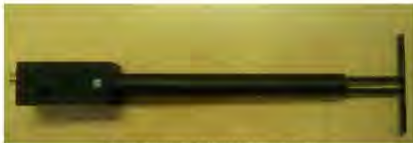
Figure 1 – MVG COMOSAR Validation Dipole
