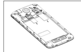
3. Insert the memory card into the card slot with the metal contacts facing down until it inserts to the right position.
