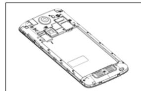
4. Insert the battery by aligning the gold contacts on the battery with the gold contacts in the battery compartment. Gently push down on the battery until it clicks into place.
