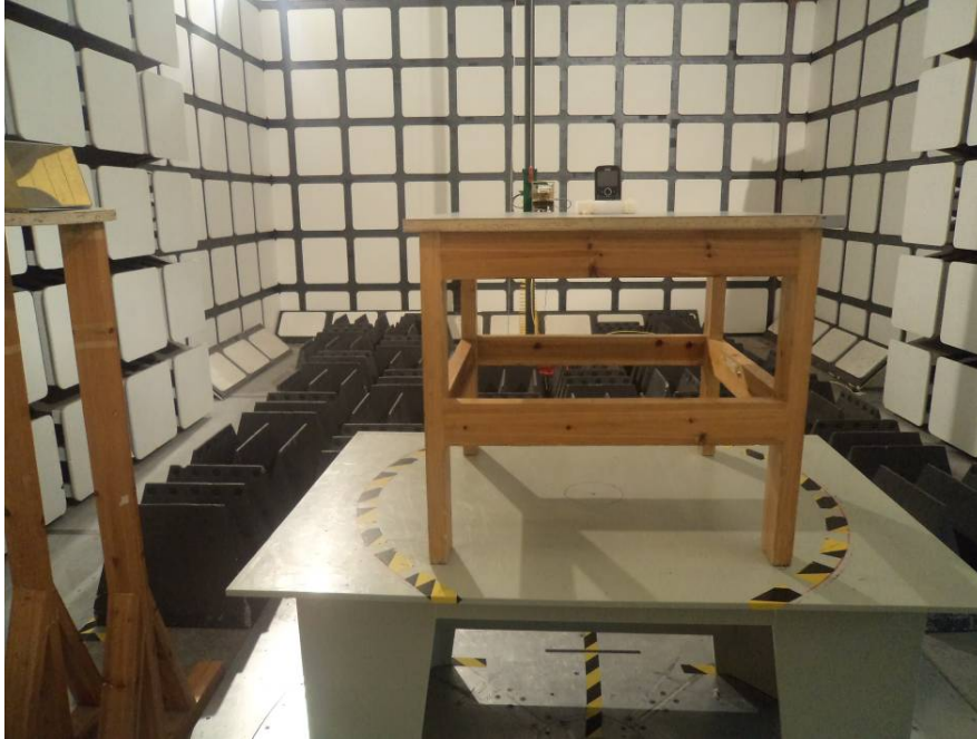
Radiated Emissions Test View
