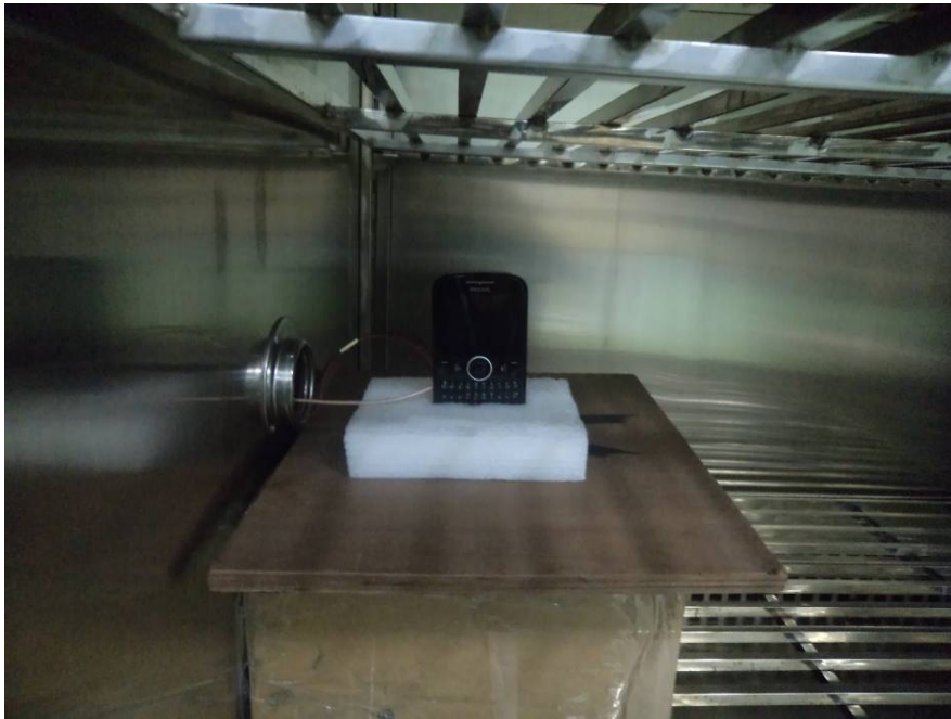
Frequency Stability Test View
