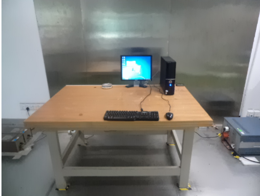
Conducted Emissions - Front View (downloading mode)
