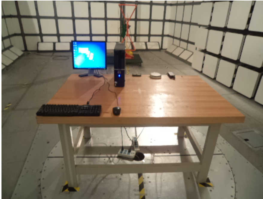
Radiated Emissions-Front View (downloading mode, 30-1000 MHz)
