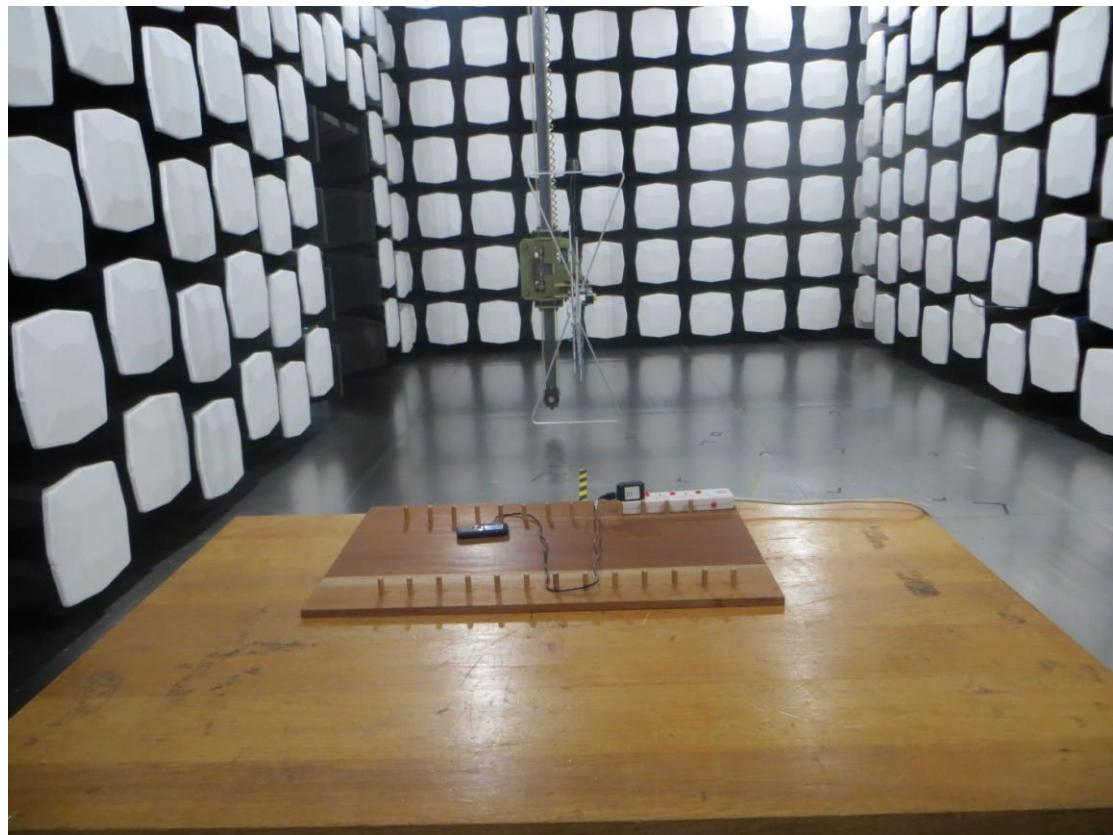
4. Part 15B Radiated emission (charger) above 1GHz
