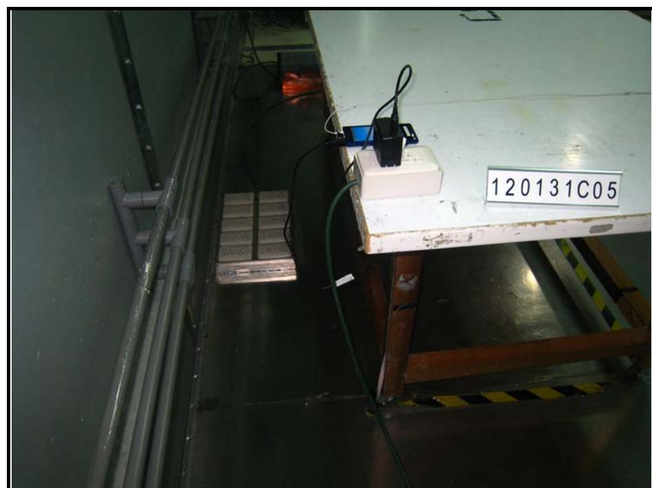
RADIATED EMISSION TEST (Z-Axis)
