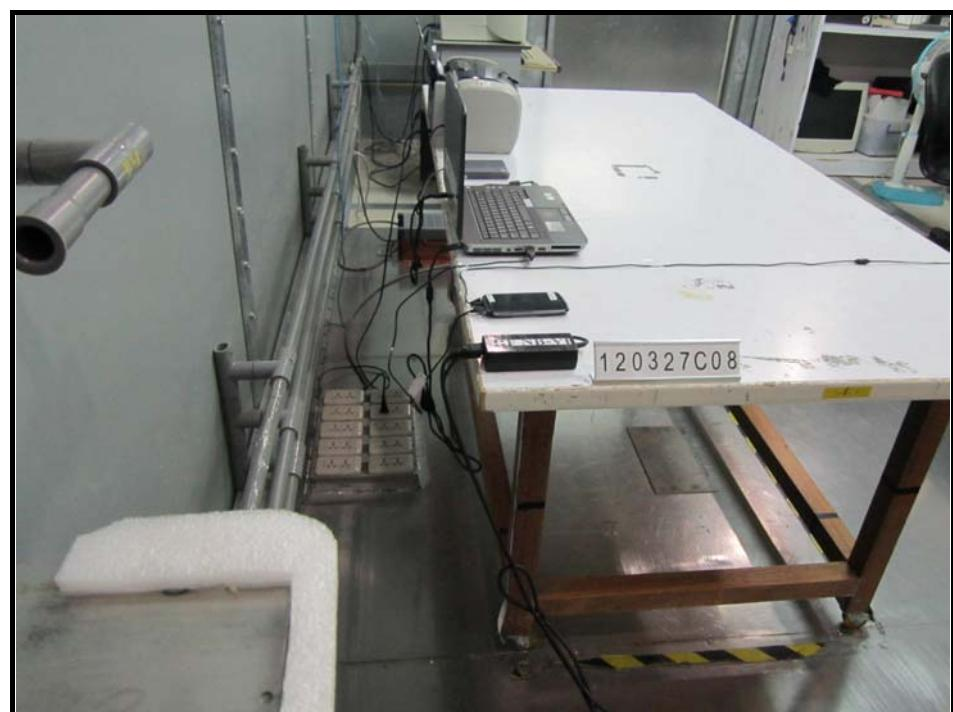
CONDUCTED EMISSION TEST (Test Mode D)
