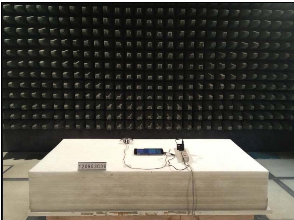
RADIATED EMISSION TEST (Test Mode B)
