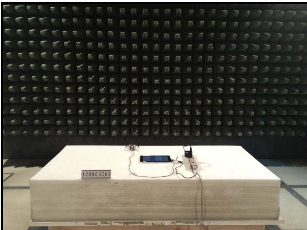
RADIATED EMISSION TEST (Test Mode B)
