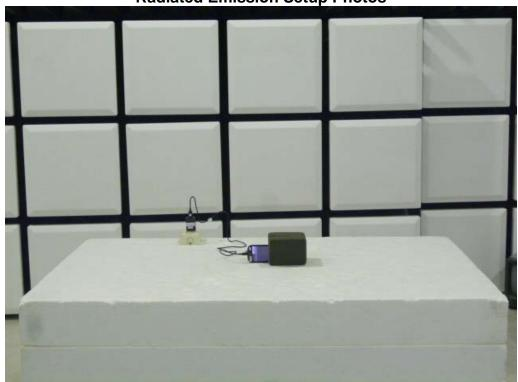
Radiated Emission Setup Photos (10~30MHz)
