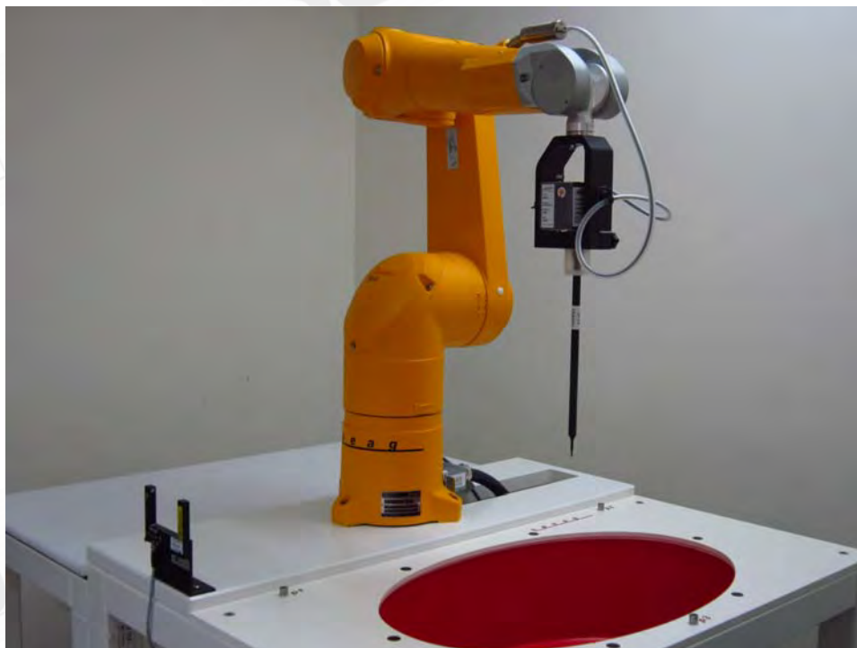
Fig.1 Photograph of the SAR measurement system
