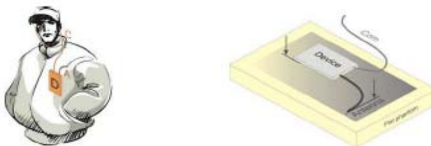
Fig. 11: Measurement position for clothing integrated devices.
