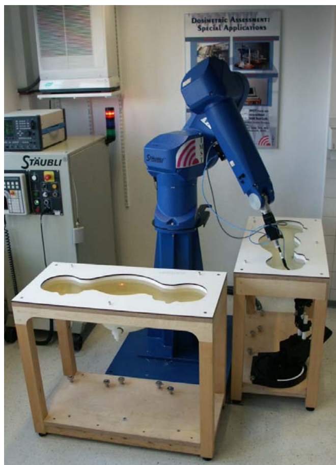
Fig. 14: The measurement set-up with two phantoms containing tissue simulating liquid.
