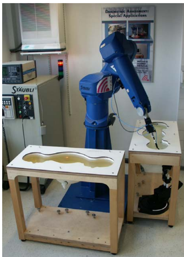
Fig. 8: The measurement set-up with two phantoms containing tissue simulating liquid.
