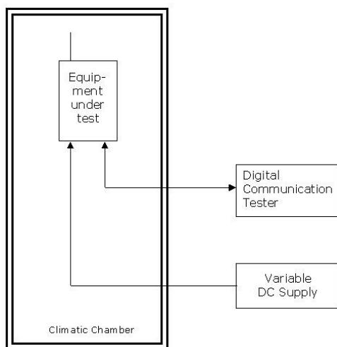
Principle set-up for tests under extreme test conditions
