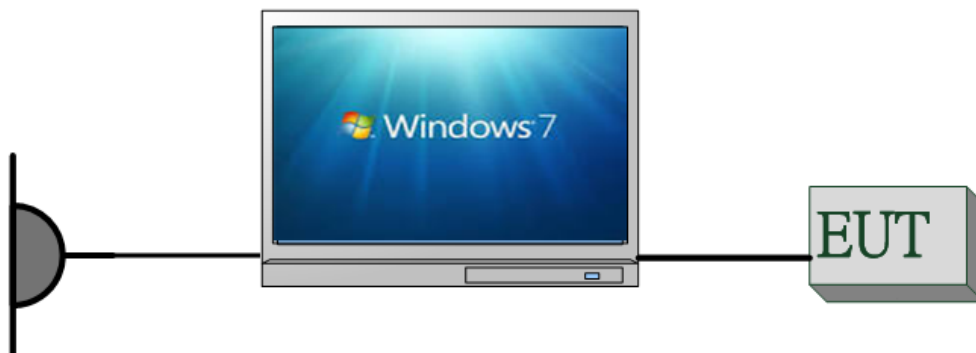
Fig. 2-1 Radiated Emission & Conducted (Antenna Port) Configuration
