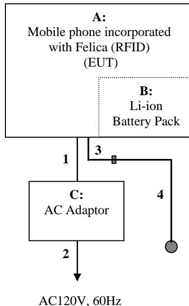
Note: EUT has one connector which can be connected either AC adapter ( No.1 above) or Earphone ( No. 3 above). On each tests, the result of the worse condition is reported as worst case in this report.
