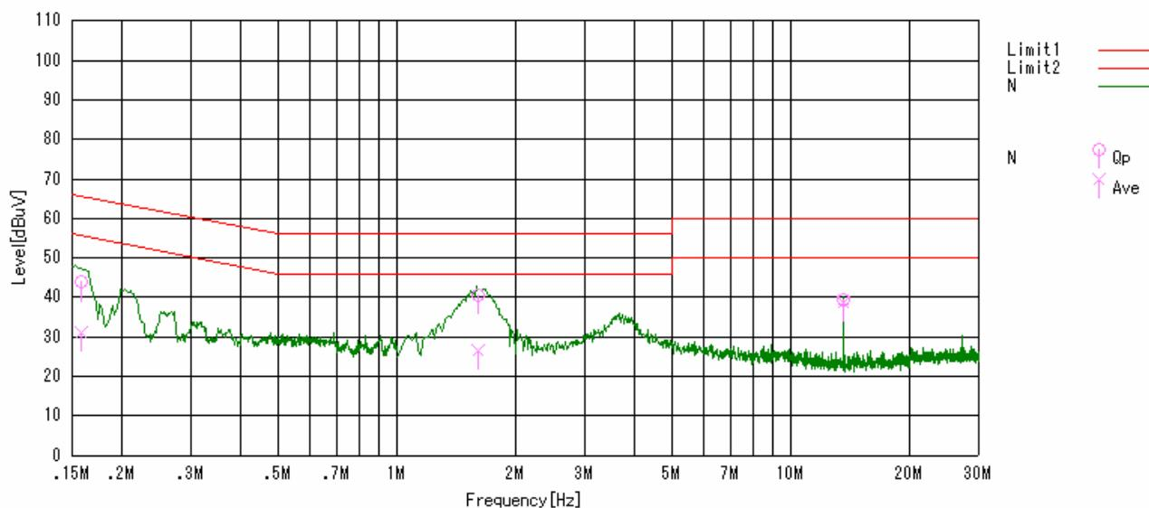
**AC Power line conducted emission. (Phase L)**
