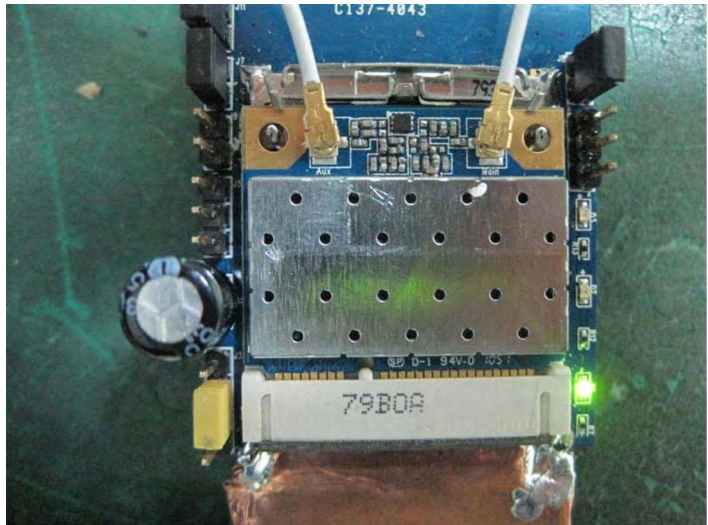
**Configuration 2 with Ant. 2 (Dipole Antenna)**
