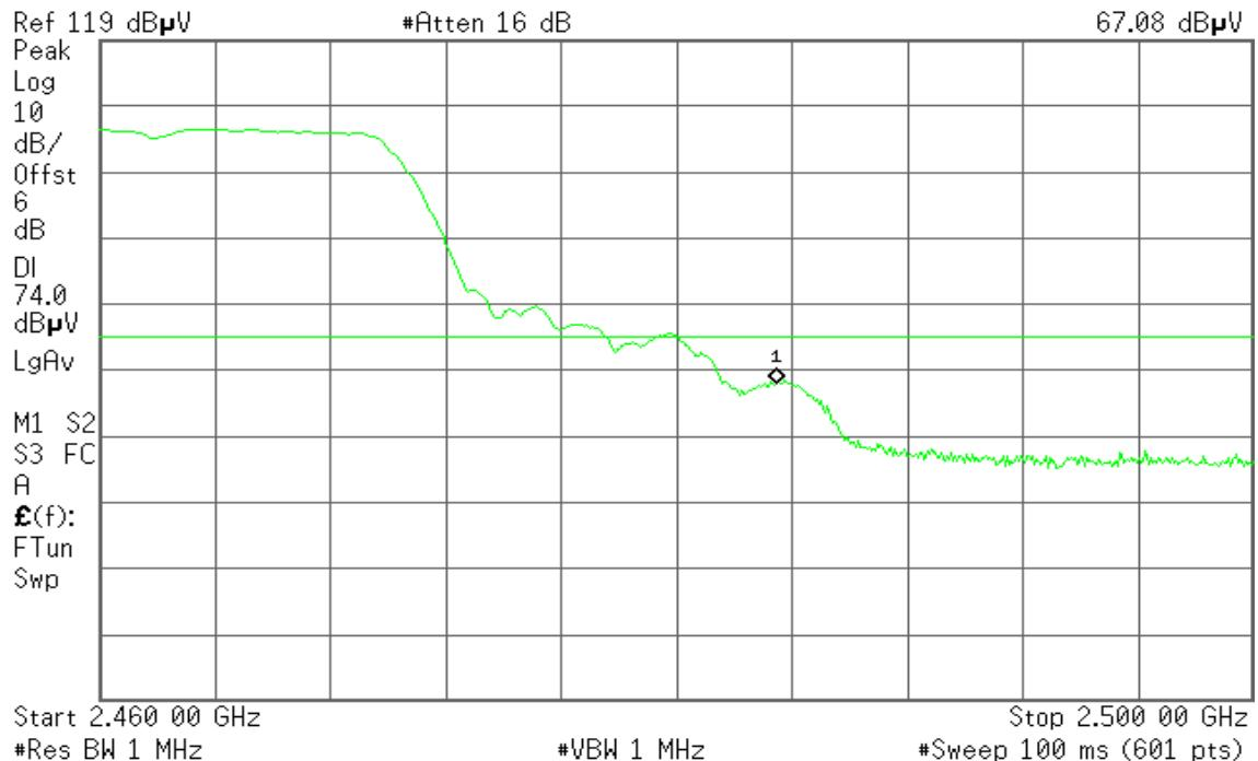
**Detector mode: Average****Polarity: Horizontal****Agilent**
