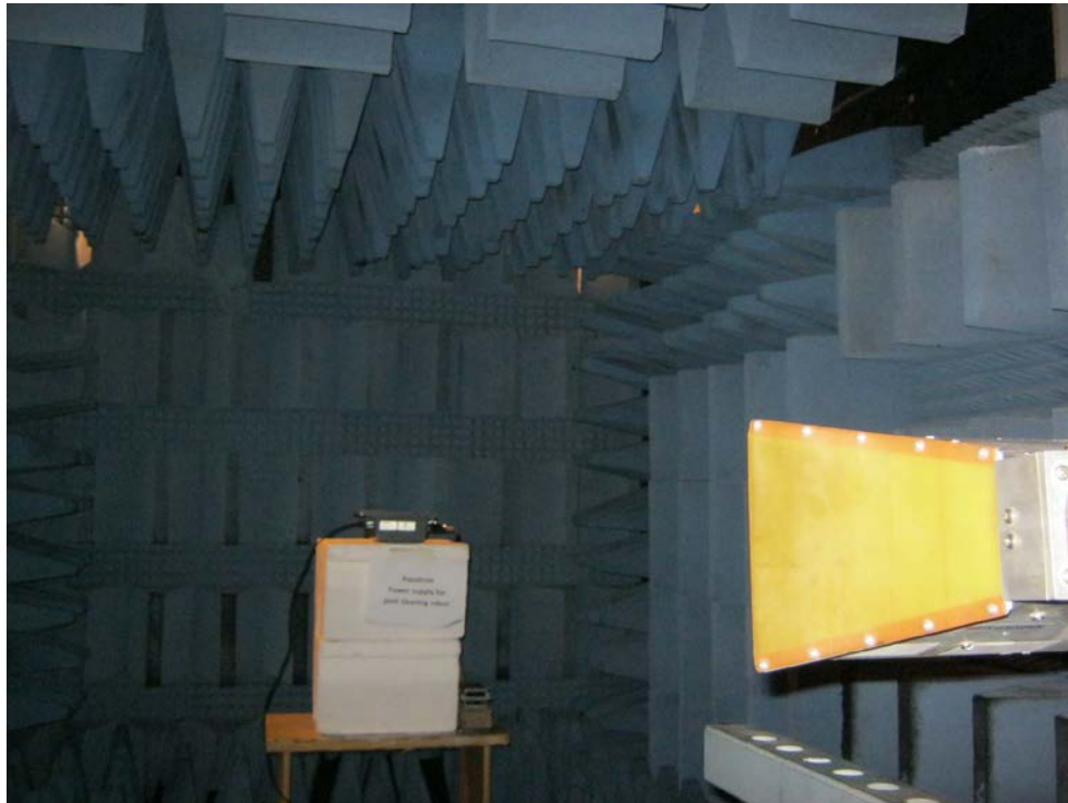
Figure 6. Radiated Emission Test
