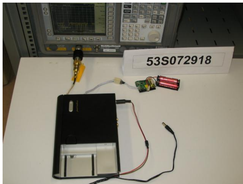
RF Conducted Spurious Emissions Test Setup
