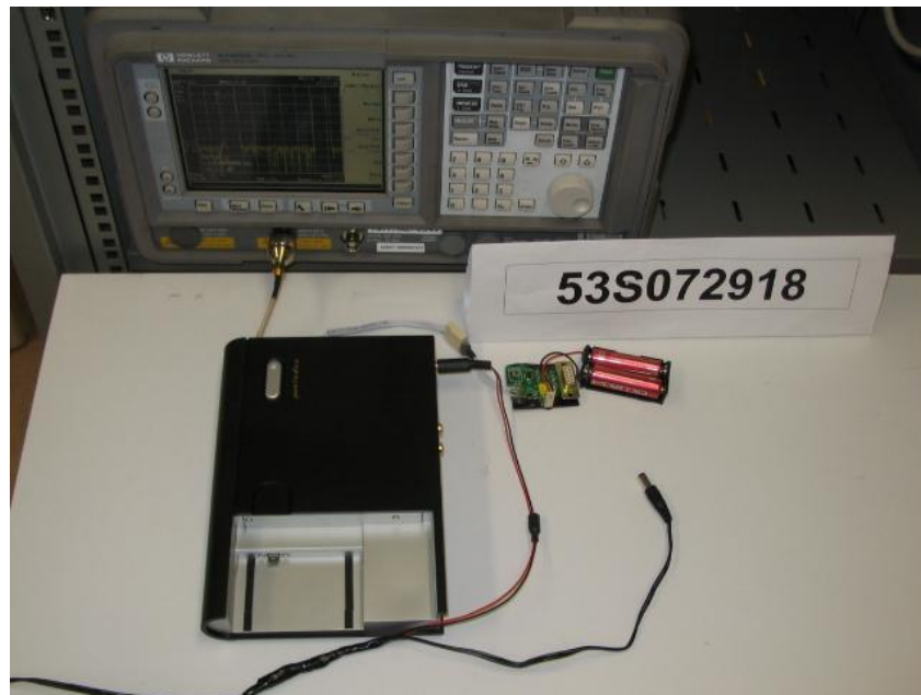
Number of Hopping Frequencies Test Setup
