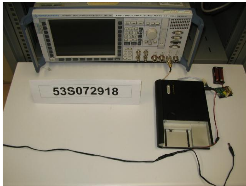
Maximum Peak Power Test Setup
