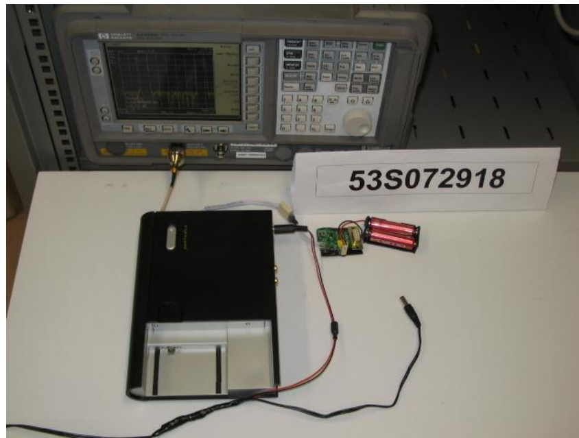
Peak Power Spectral Density Test Setup
