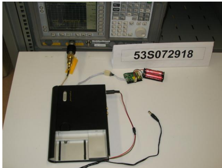
Band Edge Compliance (Conducted) Test Setup
