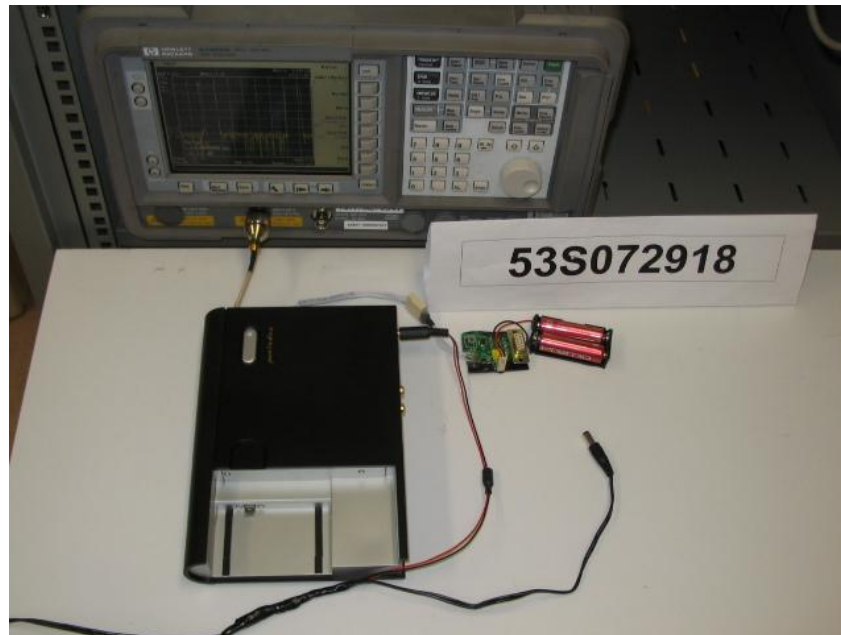
Carrier Frequency Separation Test Setup
