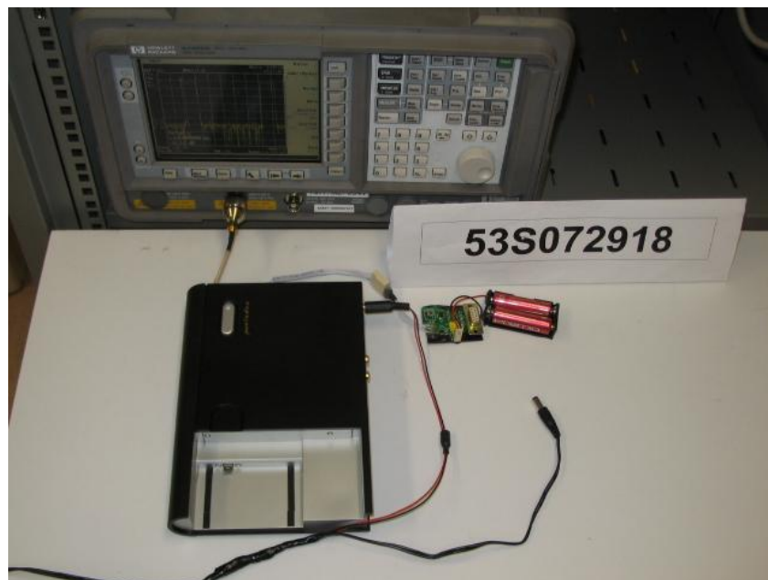
Spectrum Bandwidth (20dB Bandwidth Measurement) Test Setup
