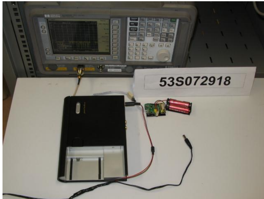
Average Frequency Dwell Time Test Setup
