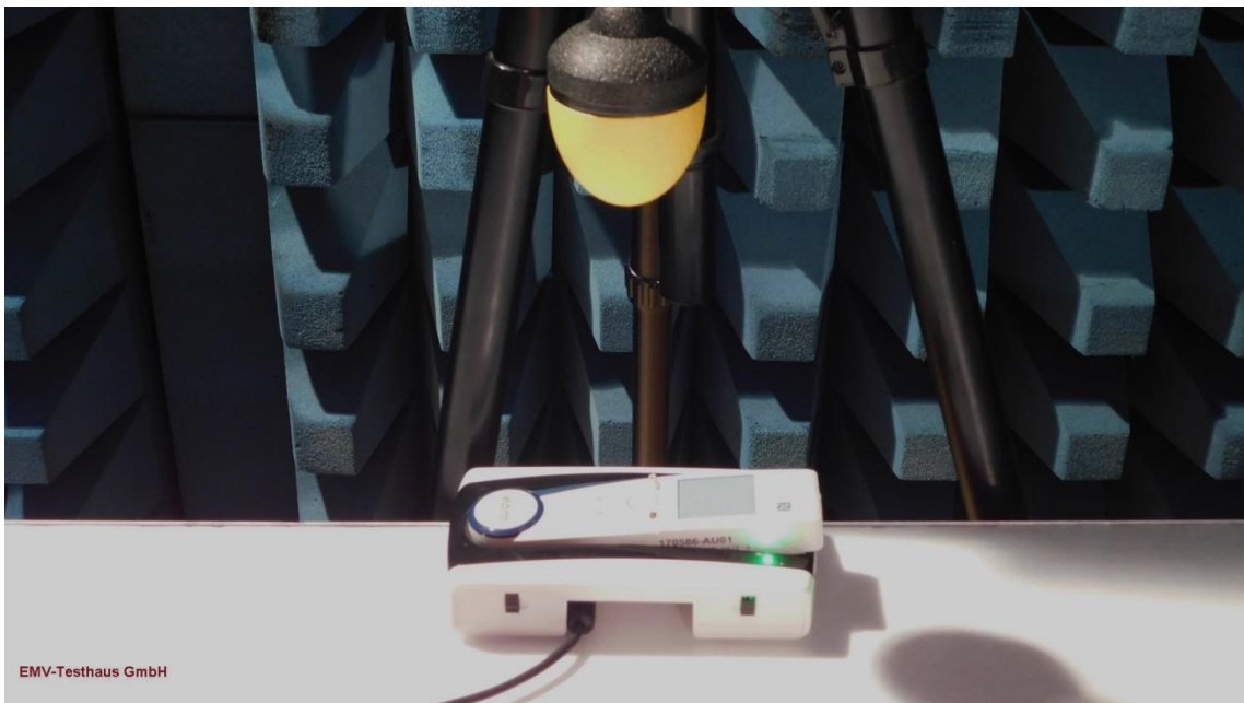
Picture 2: Setup of electric field test for charging mode
