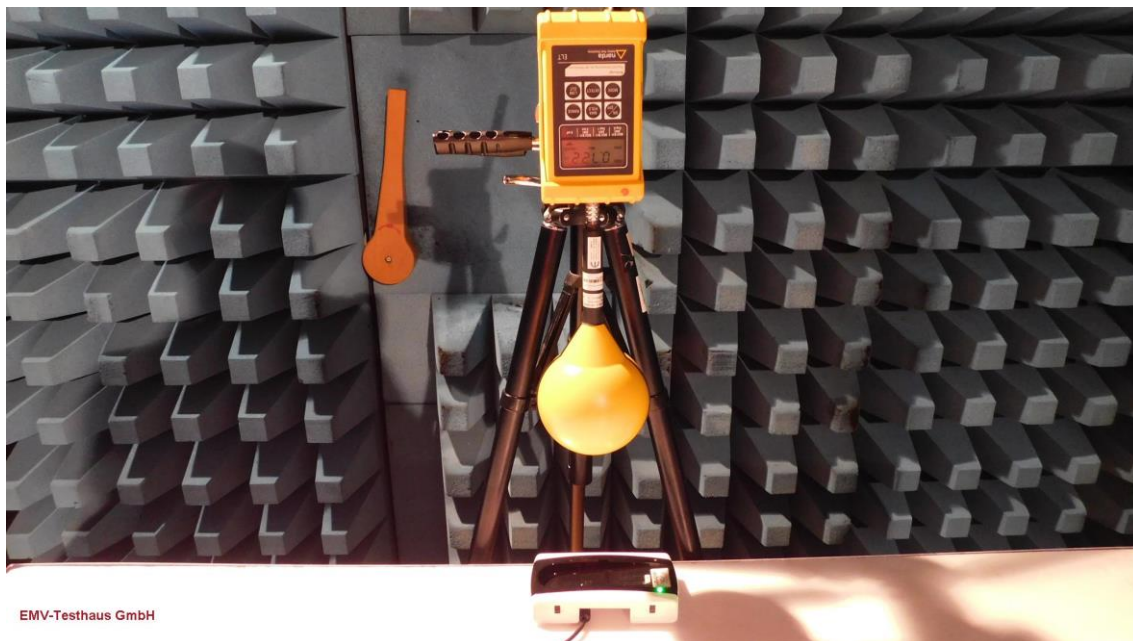
Picture 3: Setup of magnetic field test for standby mode
