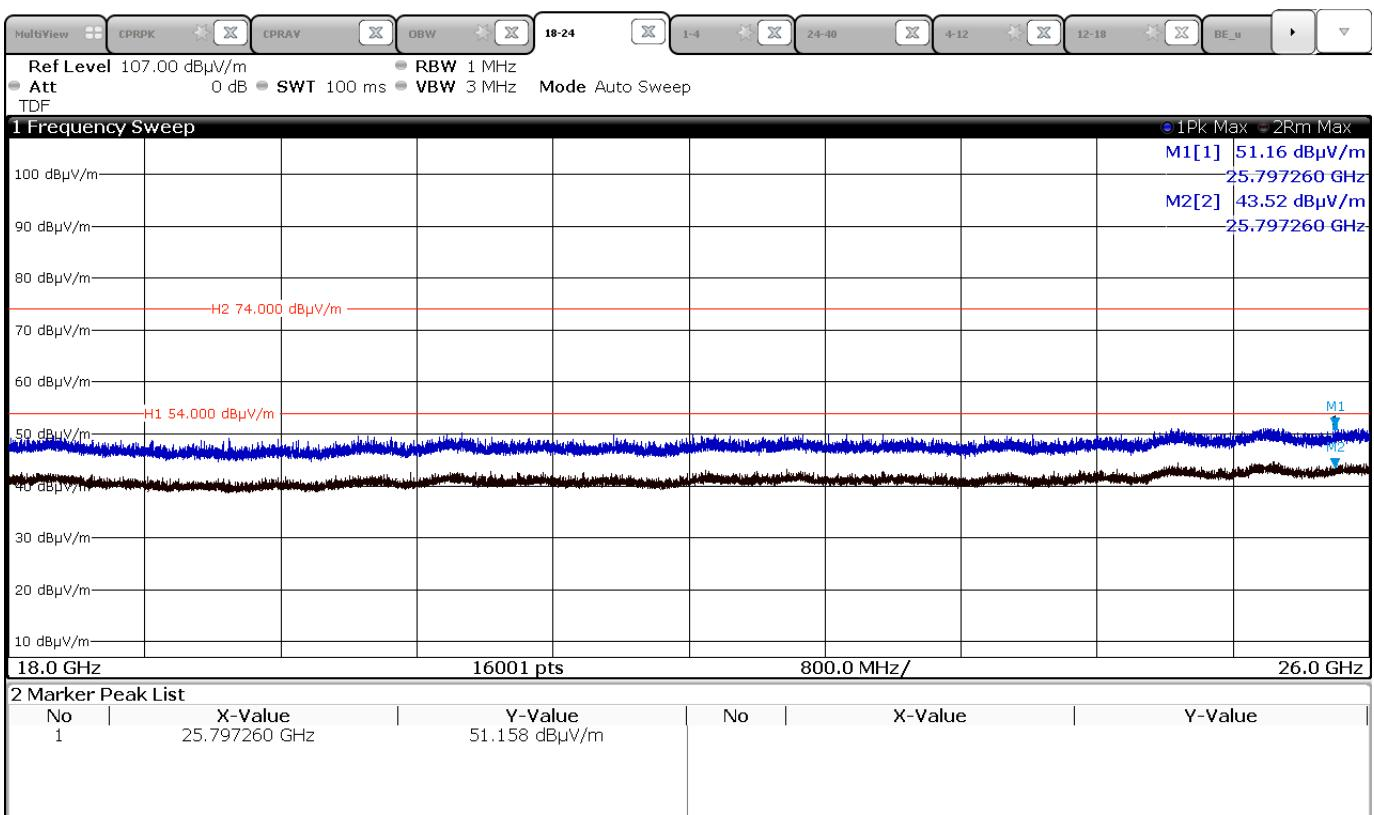
Radiated limits according to FCC Part 15 Section 15.209(a) for spurious emissions which fall in restricted bands:
