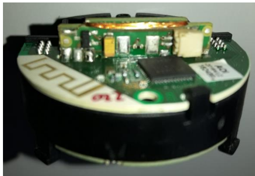
old wired RFID antenna
