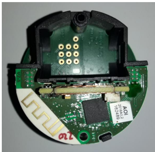
old wired RFID antenna
