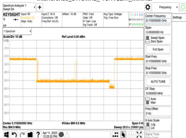
802.11ax_80MHz_CF 6145MHz_ Interference_6110MHz_-70.69dBm_Normal
