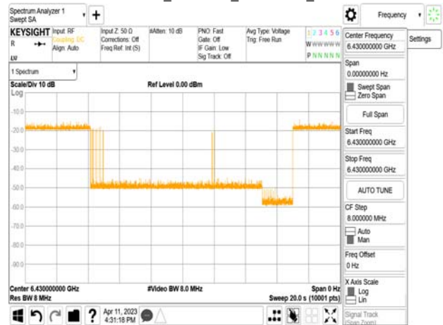
802.11ax_80MHz_CF 6465MHz_ Interference_6430MHz_-68.68dBm_Normal
