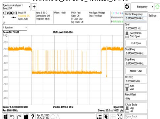
802.11ax_80MHz_CF 6705MHz_ Interference_6670MHz_-76.7dBm_Normal
