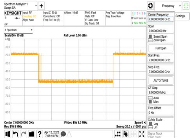
802.11ax_80MHz_CF 7025MHz_ Interference_7060MHz_-74.61dBm_Normal
