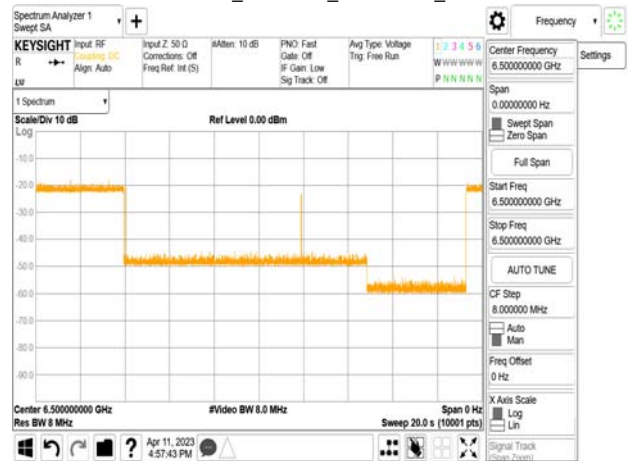
802.11ax_80MHz_CF 6465MHz_ Interference_6500MHz_-67.66dBm_Normal
