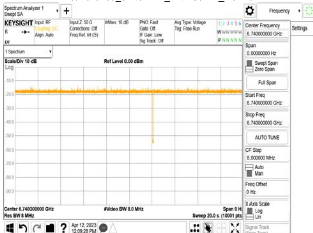
802.11ax_80MHz_CF 6705MHz_ Interference_6740MHz_-74.73dBm_Normal
