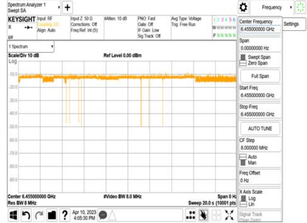
802.11ax_20MHz_CF 6455MHz_ Interference_6455MHz_-70.62dBm_Normal
