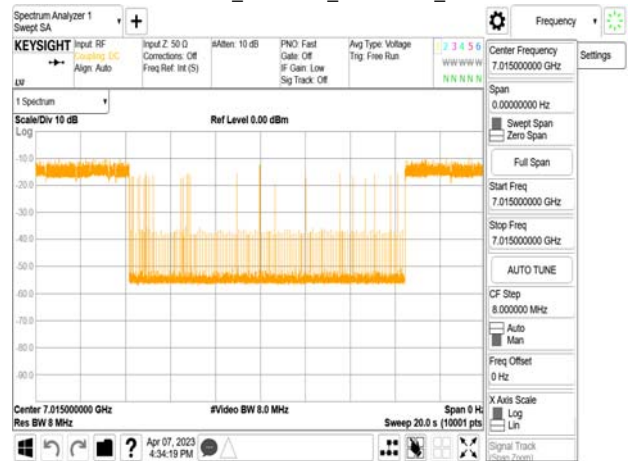
802.11ax_20MHz_CF 7015MHz_ Interference_7015MHz_-76.62dBm_Normal
