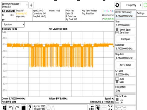
802.11ax_80MHz_CF 6705MHz_ Interference_6740MHz_-73.66dBm_Normal
