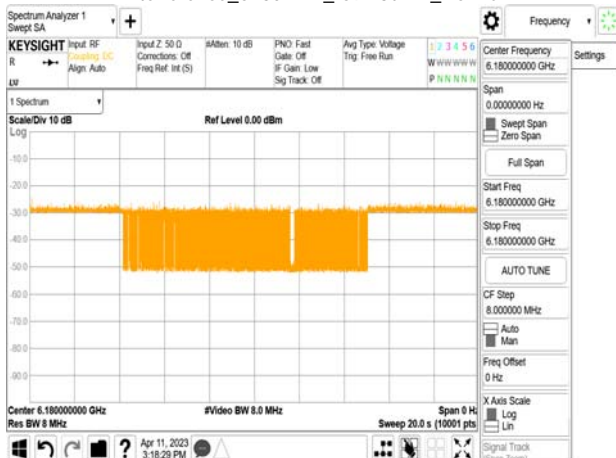
802.11ax_80MHz_CF 6145MHz_ Interference_6180MHz_-69.73dBm_Normal
