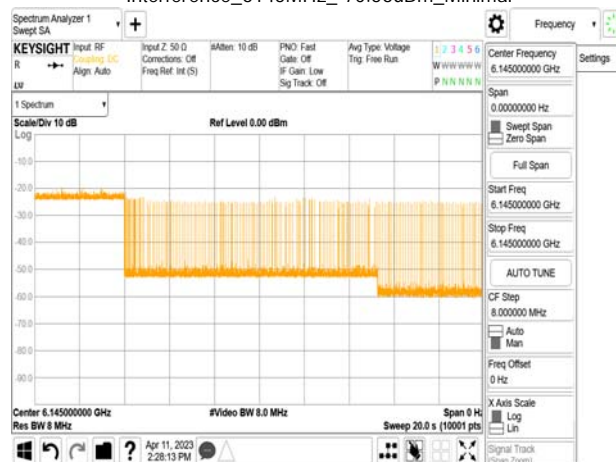
802.11ax_80MHz_CF 6145MHz_ Interference_6145MHz_-73.56dBm_Normal
