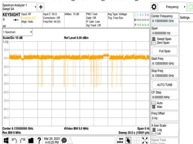
802.11ax_20MHz_CF 6135MHz_ Interference_6135MHz_-73.83dBm_Normal
