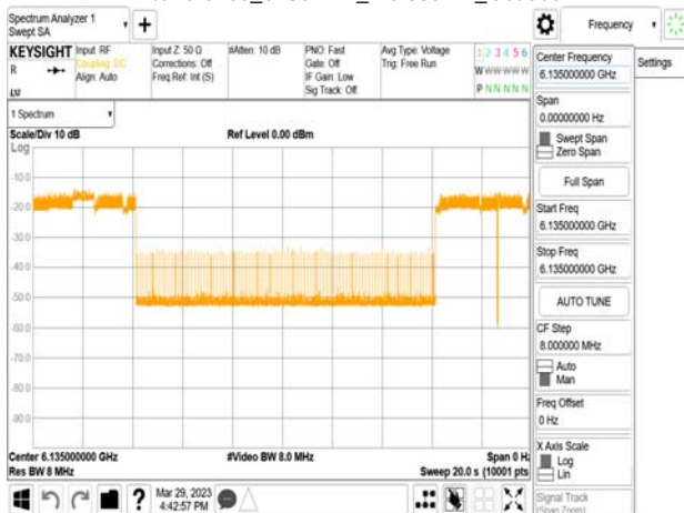
802.11ax_20MHz_CF 6135MHz_ Interference_6135MHz_-71.83dBm_Minimal
