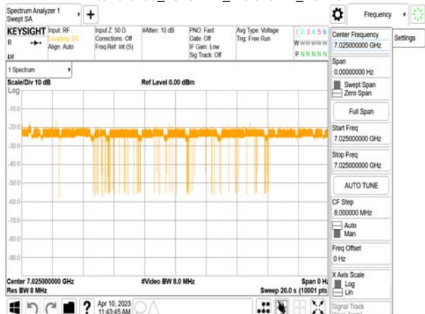
802.11ax_80MHz_CF 7025MHz_ Interference_7025MHz_-76.52dBm_Normal
