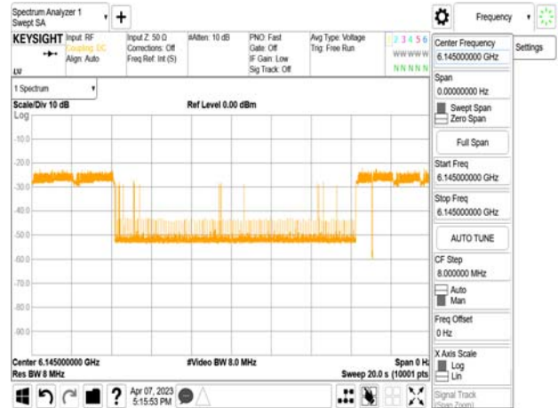
802.11ax_80MHz_CF 6145MHz_ Interference_6145MHz_-73.65dBm_Normal
