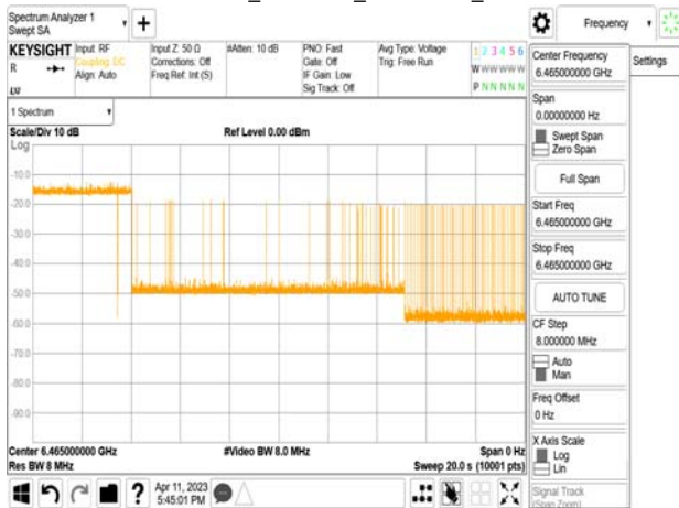
802.11ax_80MHz_CF 6465MHz_ Interference_6465MHz_-70.85dBm_Normal
