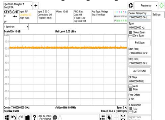
802.11ax_80MHz_CF 7025MHz_ Interference_7060MHz_-74.61dBm_Normal
