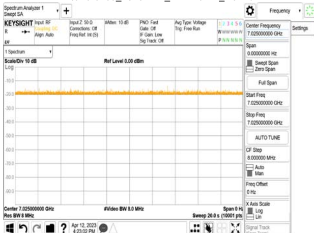
802.11ax_80MHz_CF 7025MHz_ Interference_7025MHz_-77.72dBm_Normal
