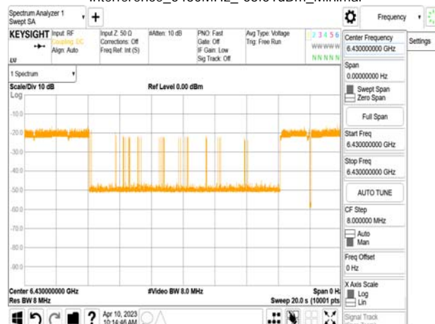
802.11ax_80MHz_CF 6465MHz_ Interference_6430MHz_-70.61dBm_Normal
