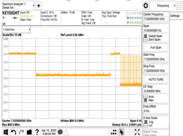
802.11ax_80MHz_CF 7025MHz_ Interference_7025MHz_-74.72dBm_Minimal
