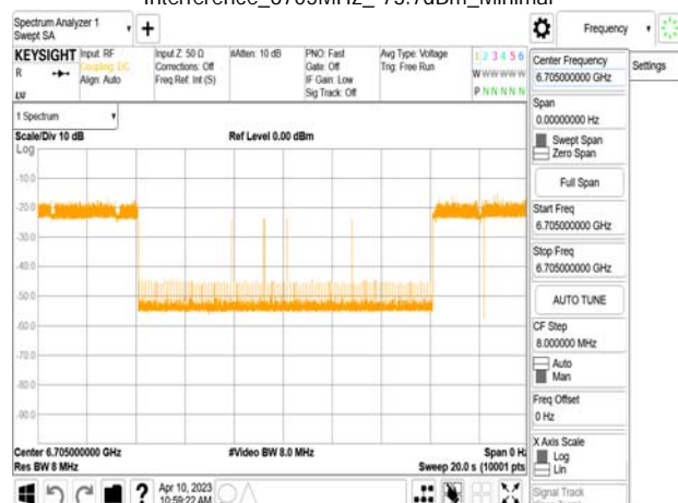
802.11ax_80MHz_CF 6705MHz_ Interference_6705MHz_-76.7dBm_Normal
