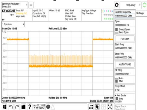
802.11ax_20MHz_CF 6695MHz_ Interference_6695MHz_-74.74dBm_Minimal
