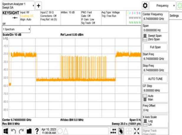
802.11ax_80MHz_CF 6705MHz_ Interference_6740MHz_-73.66dBm_Normal
