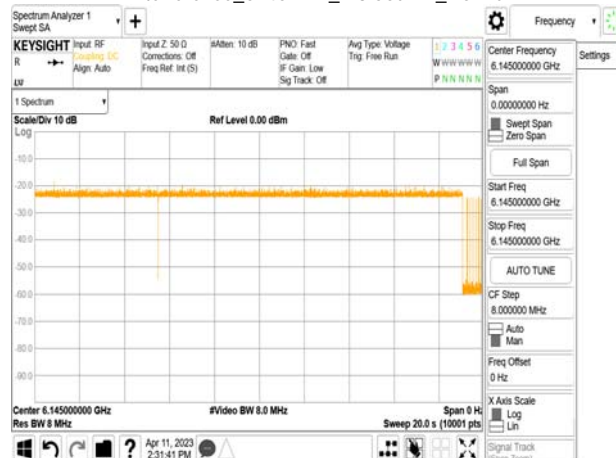
802.11ax_80MHz_CF 6145MHz_ Interference_6145MHz_-73.56dBm_Normal
