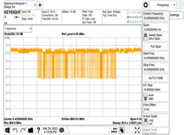
802.11ax_20MHz_CF 6455MHz_ Interference_6455MHz_-70.64dBm_Normal
