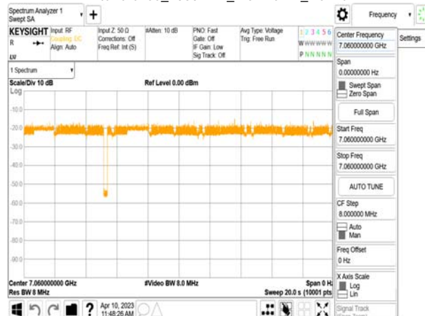
802.11ax_80MHz_CF 7025MHz_ Interference_7060MHz_-76.77dBm_Normal
