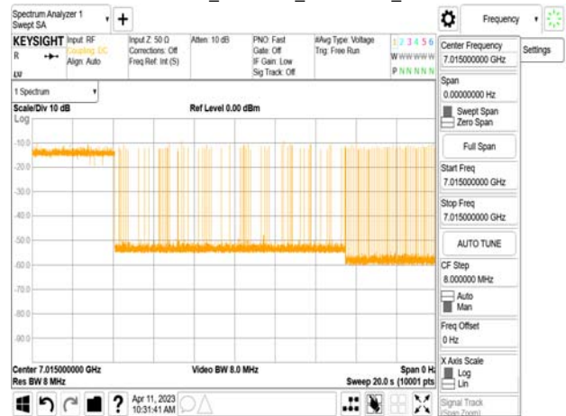
802.11ax_20MHz_CF 7015MHz_ Interference_7015MHz_-76.52dBm_Normal
