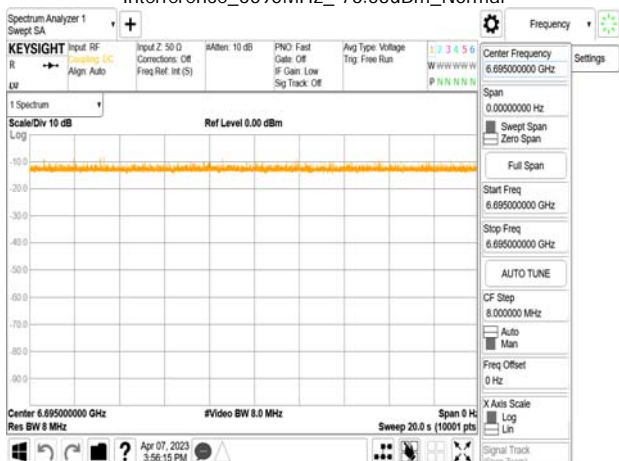
802.11ax_20MHz_CF 6695MHz_ Interference_6695MHz_-76.53dBm_Normal
