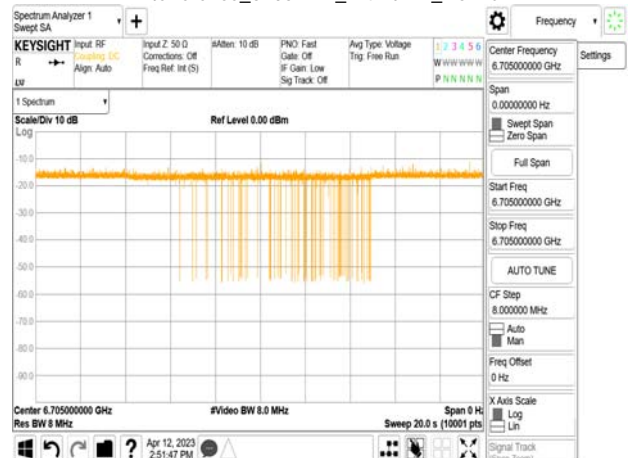
802.11ax_80MHz_CF 6705MHz_ Interference_6705MHz_-74.7dBm_Normal
