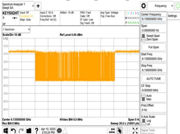
802.11ax_20MHz_CF 6135MHz_ Interference_6135MHz_-72.57dBm_Normal
