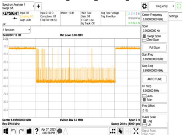
802.11ax_20MHz_CF 6695MHz_ Interference_6695MHz_-76.53dBm_Normal
