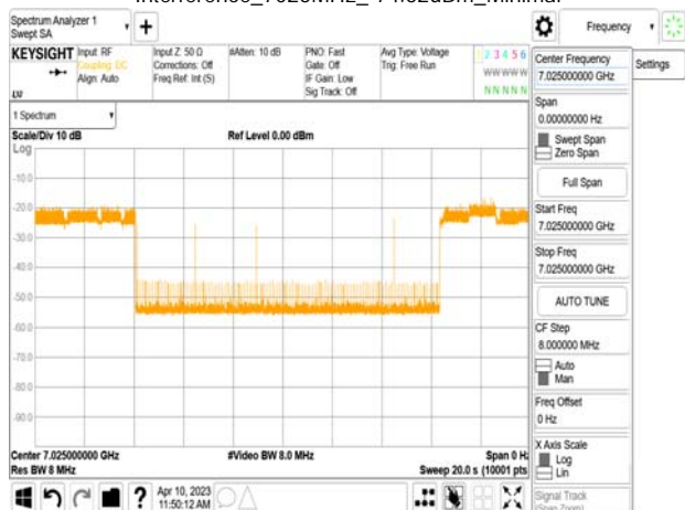
802.11ax_80MHz_CF 7025MHz_ Interference_7025MHz_-76.52dBm_Normal
