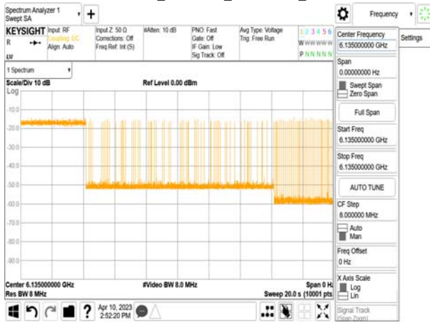
802.11ax_20MHz_CF 6135MHz_ Interference_6135MHz_-72.57dBm_Normal
