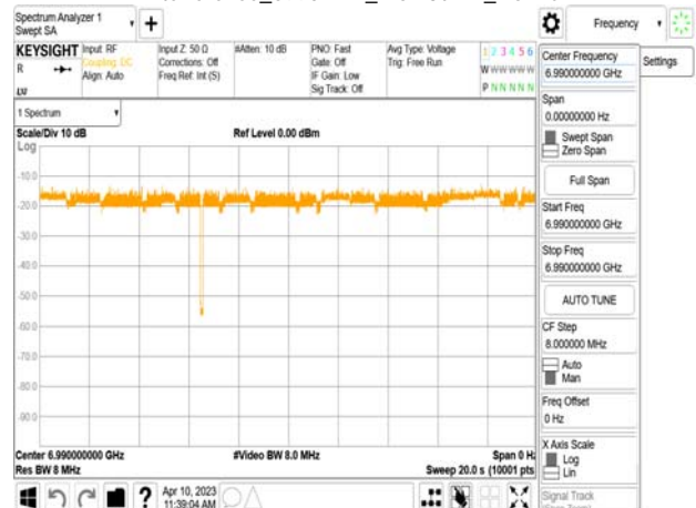
802.11ax_80MHz_CF 7025MHz_ Interference_6990MHz_-76.73dBm_Normal
