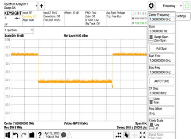
802.11ax_80MHz_CF 7025MHz_ Interference_7060MHz_-72.61dBm_Minimal
