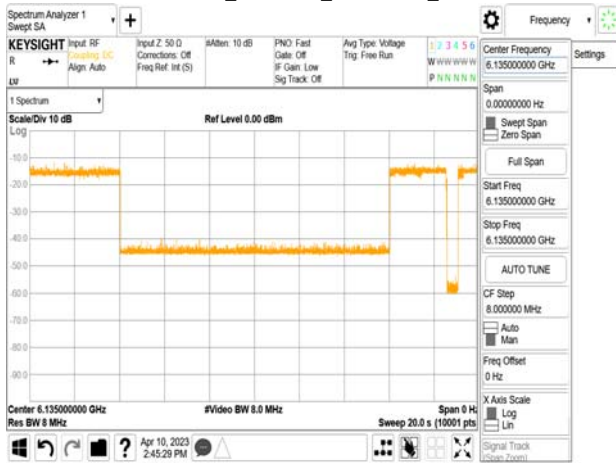
802.11ax_20MHz_CF 6135MHz_ Interference_6135MHz_-69.57dBm_Minimal
