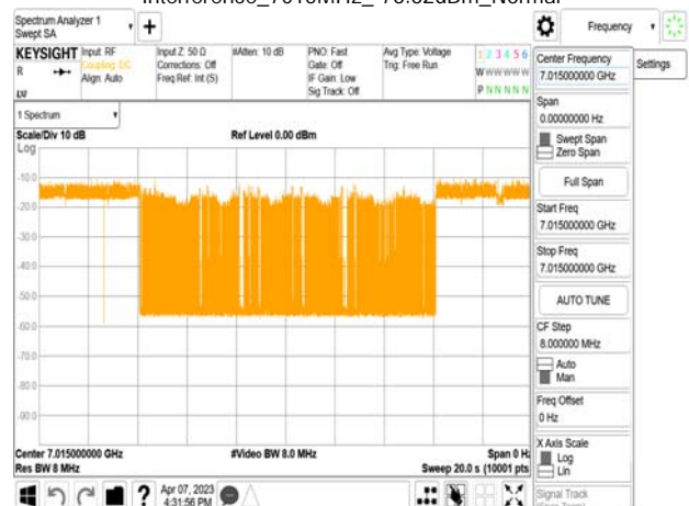
802.11ax_20MHz_CF 7015MHz_ Interference_7015MHz_-76.62dBm_Normal
