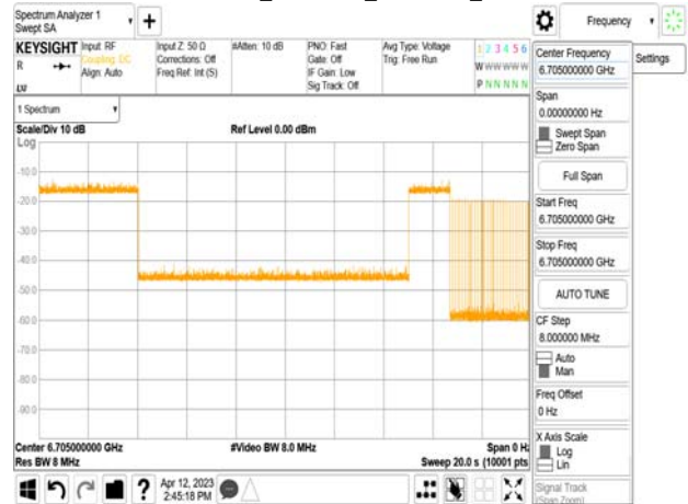
802.11ax_80MHz_CF 6705MHz_ Interference_6705MHz_-71.7dBm_Minimal
