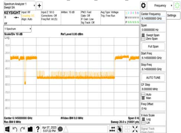
802.11ax_80MHz_CF 6145MHz_ Interference_6145MHz_-71.15dBm_Minimal
